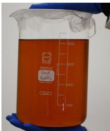
Figure 36 4 litres of BNC solution made using sericin extract and AgNO 3 .
