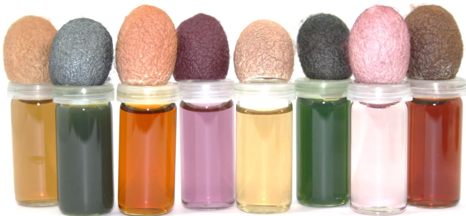
Figure 14 Colloidal solutions and the relevant soft bioshells decorated with silver and gold nanoparticles thereby shining in miscellaneous plasmonic colors.
