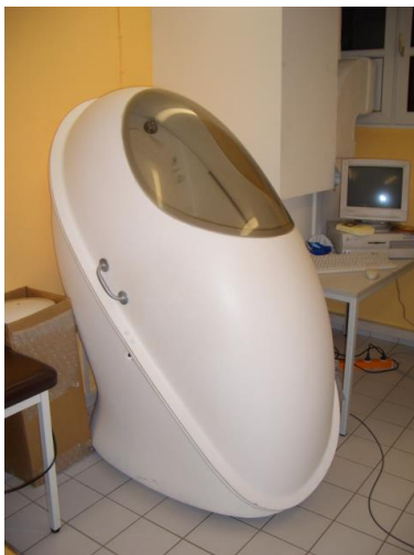
Abbildung 2 Air-Displacement-Plethysmograph (BOD POD®-Body Composition System; Life Measurement, Inc., Concord, Kalifornien, USA)
