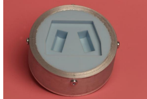
Fig. 8 – The aluminum custom flask (left)
