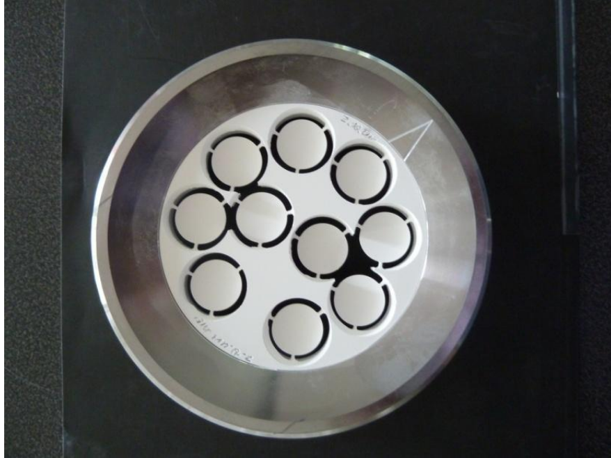
Figure 3: Close-up of blank after milling the discs
