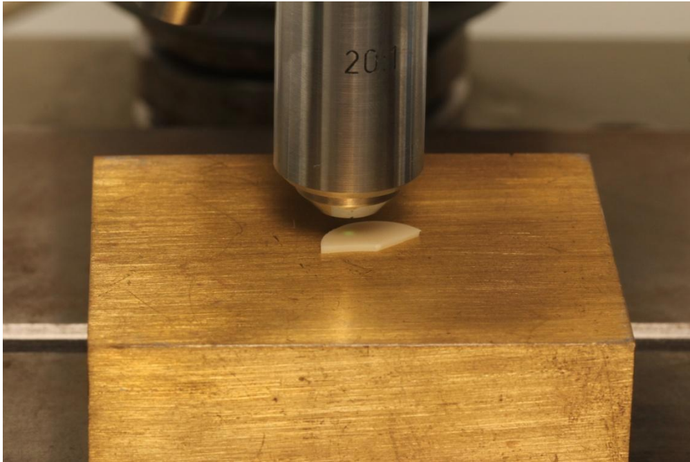
Figure 18: Observation of indentation under 20× magnification
