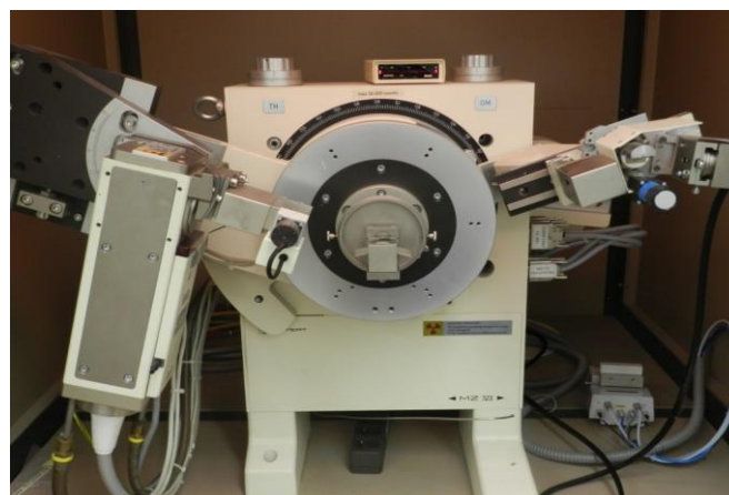
Figure 12: X-ray source, disc and receptor
