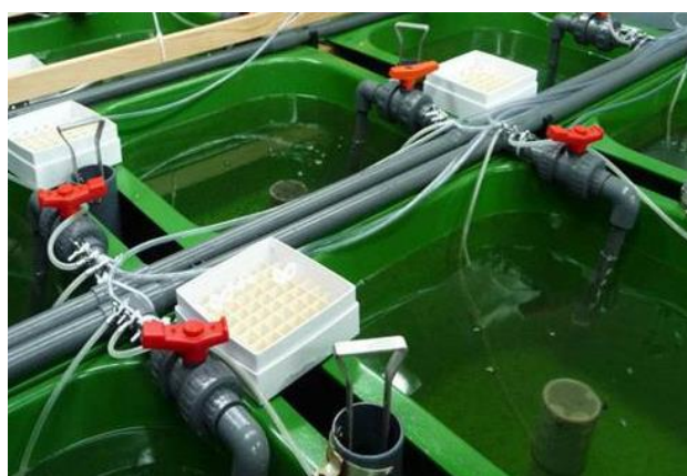
Fig. 6. Experimental 60 L tanks for immunostimulation experiments in sea bass larvae and juveniles.
