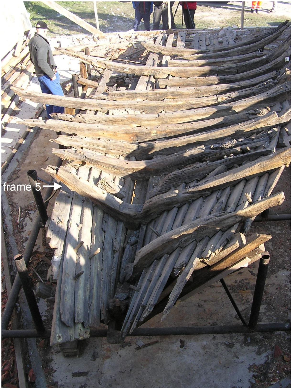
Fig. 6-4. This photo shows the inner part, featuring the bilge-well and frame 5 (Photo: Vello Mäss, modified by the author).
