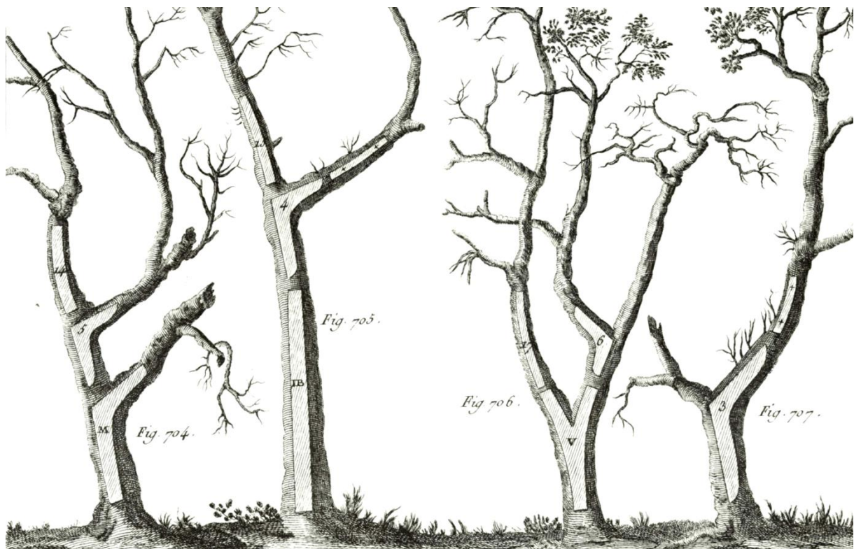
Fig. 5-1. This 18 th century naval architectural manual exemplifies how to make best use of branches for compass timber. The trees were apparently pruned to control their growth. While these specimens would have been perfect sources for structural timber, most of them would have been very poor choices for planks (Source: Panckoucke et al. 1786, pl. 103).
