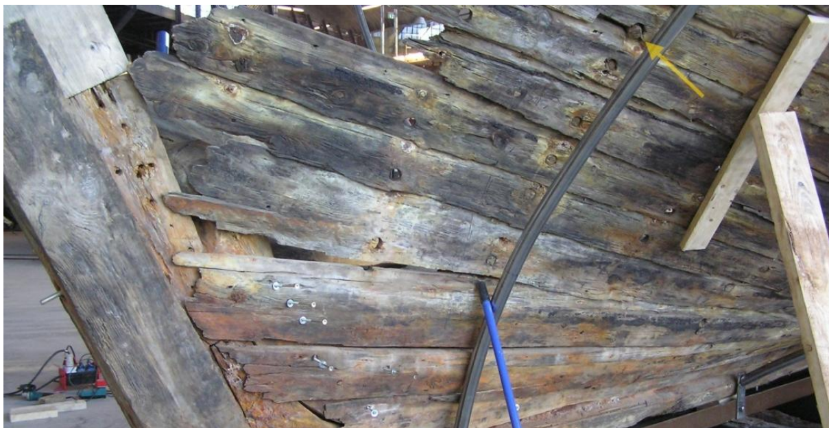
Fig. 6-6. Some of the treenail holes were drilled through the land, often directly at the edge of the plank, as the yellow arrow indicates (Photo: Vello Mäss, modified by the author).
