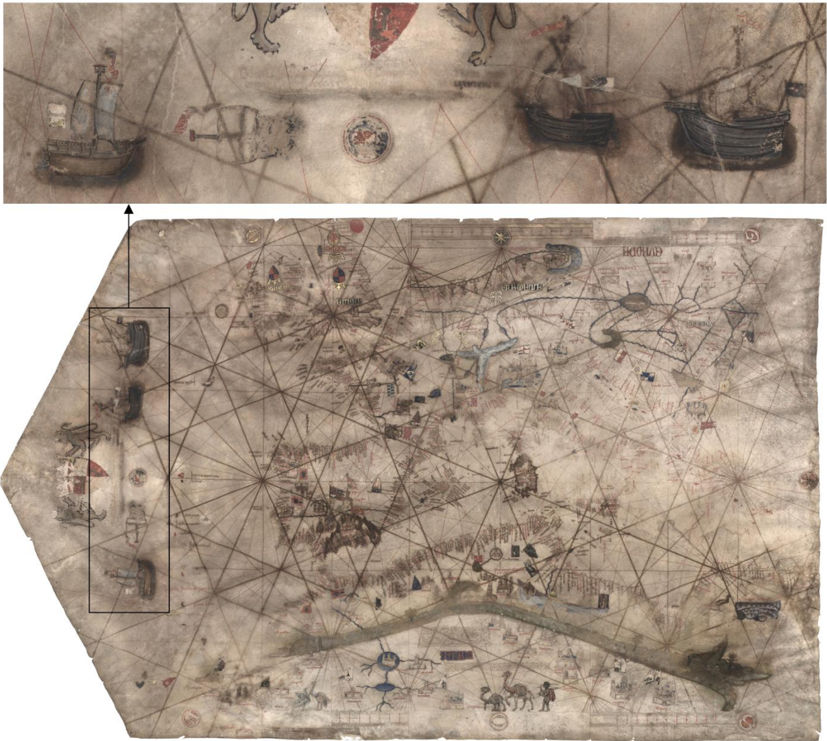
Fig. 6. Ship depictions on an excerpt – from the left side – of Becharius's portolan chart of 1426, showing three square-rigged ships of which one – on the right side – also carried a lateen-rigged mizzen mast. Also the portolan itself is interesting: Note the astounding accuracy of the coastlines of the Mediterranean, Atlantic coast and the English Canal in contrast to the area beyond Flanders, where the accuracy ends abruptly. On the one hand this can be attributed to the extensive Mediterranean-Flemish trade and on the other hand to the scientific navigation method employed by the Italians, through which the coastline could be mapped accurately (Source: Bavarian State Library).
