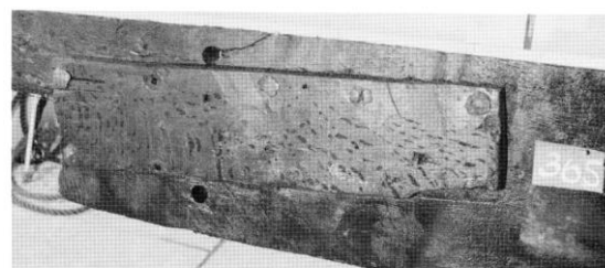
Fig. 5-12. Mended part in the Bremen Ship’s (1378) planking: Patched over crack (top) and bung (left) (Photos: Lahn 1992, figs. 48-49).
