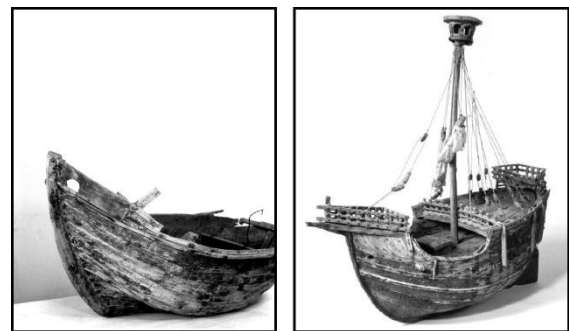
Fig. 8. Irrespective of the type-labels attached to the Ebersdorf "cog/holk" model of ca. 1400 (left) and the Mataró "carrack/nao" model from 1389-1449 (right), they appear very similar, judging from the stout impression rendered by the high freeboard, the short length-to-beam ratio and the curved stem. To contemporaries they might have appeared as a same category of ship, yet the underlying constructional principle of shell-first clinker in the former and skeleton-first carvel in the latter could not be more different (Source: left: Holger Strauß, right: Maritime Museum Rotterdam).
