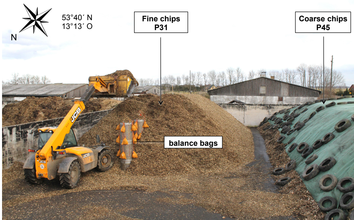
Fig. 1.2: Installation of sampling columns with balance bags during the storage intake of fine chips in a clamp silo
