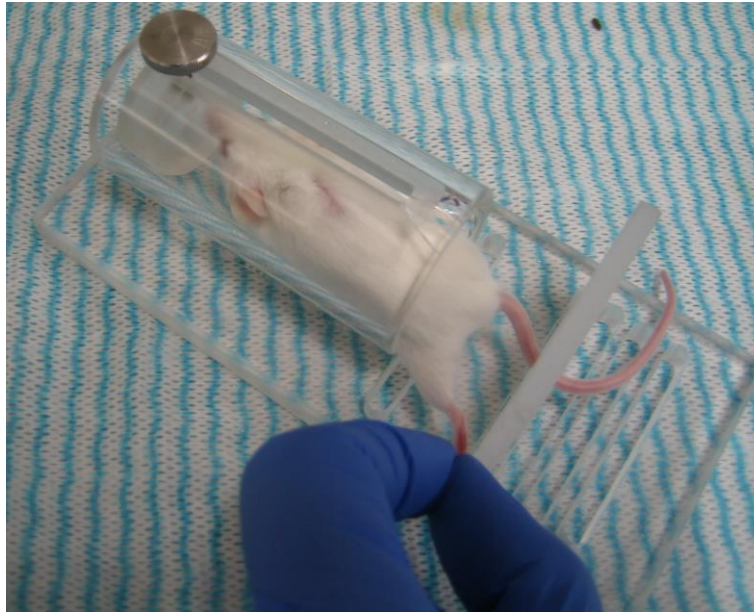
Figure 28: Custom-made mouse restrainer with a fixed test mouse. The posterior flank of the animal is accessible for irradiation.
