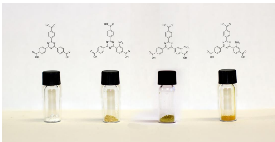
Figure S12: Differently colored triazine linkers (left: TATB-H ( 5d ); middle left: TATB-NO 2 ( meta ) ( 5b ) middle right: TATB-NO 2 ( ortho ) ( 5a ) and right: TATB-NH 2 ( meta ) ( 5c )).
