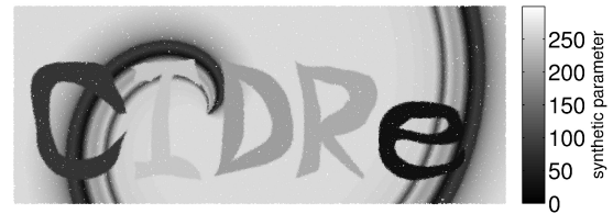
Figure 22: Central part of synthetic data set with coordinates in a range of 1 \leq X \leq 500 and 200 \leq Y \leq 400 . For validation, the complete synthetic data set was used, which contains 500 000 randomly scattered data points. The data parameter is based on the gray levels of the original raster image (Figure 21).
