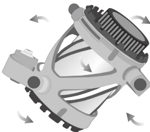
Figure 3-14 Rotational movement of the Turbula blender
