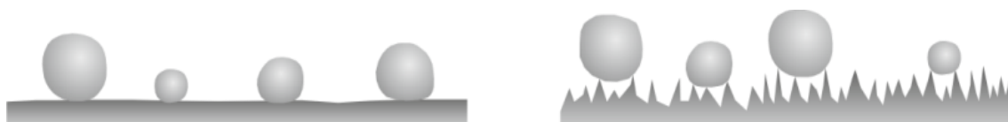
Figure 4-33 Schematic illustration of a plain untreated GB surface (left) and a surface subjected to TC milling (right) occupied with spray-dried API particles
