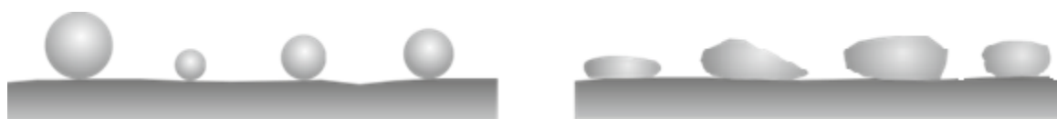
Figure 4-53 Schematic illustration of plain untreated GB surfaces occupied with spherical spray-dried (left) and irregular shaped micronised drug particles (right)
