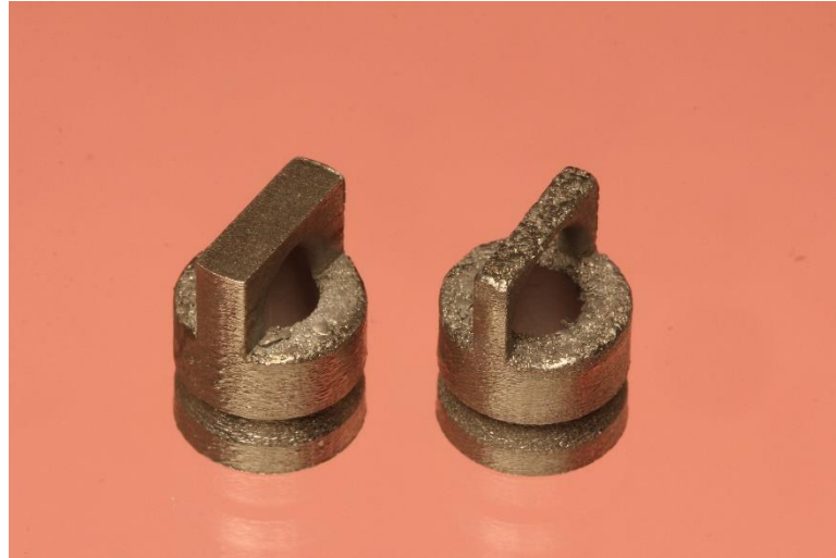
Fig. 2 – Example of a single crown ready to be cemented on the abutment. The occlusal loop was used to remove the crowns with the universal testing machine. The wider of the occlusal loops enabled chewing simulation testing.
