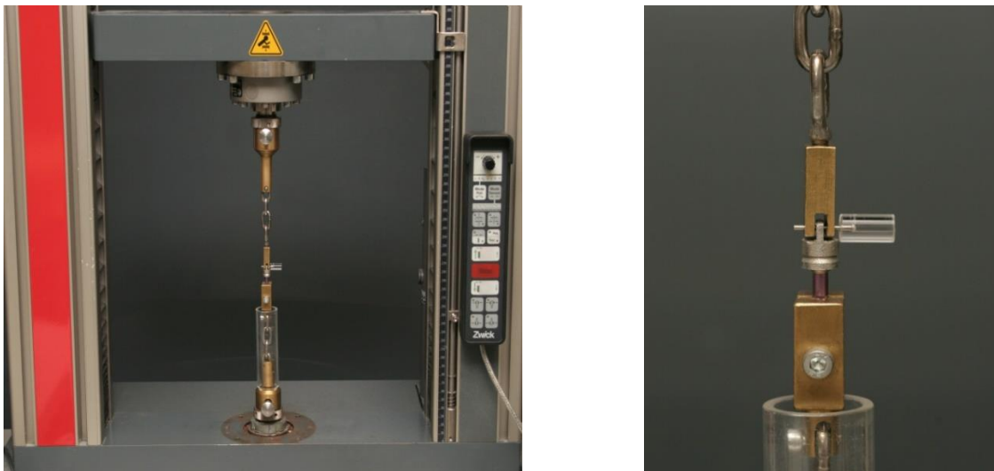
Fig. 8 – Crowns ready to be retrieved by the universal testing machine
