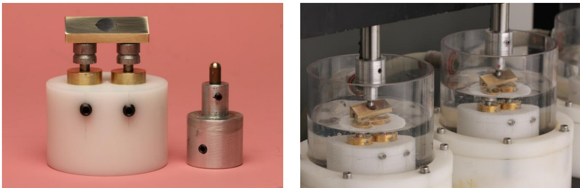
Fig. 7 – Specimens ready to be dynamically fatigued (left). Specimens inside the chewing simulator (right)
