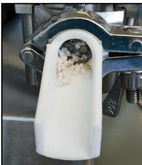
Figure IV.13. - Collection of HMG sample with the granulation heel slide.
