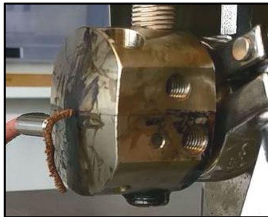
Figure IV.6. - Deteriorated extrudate strand coming out of the 2 mm standard die during an HME run.
