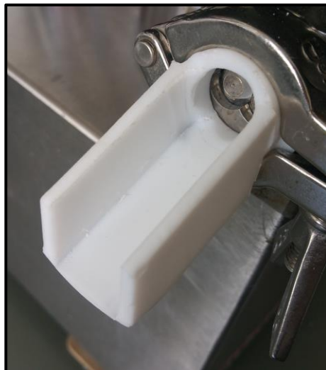
Figure III.11. - Granulation heel slide attached to the end of the Pharma 11 Twin Screw Extruder barrel.
