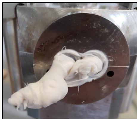
Figure IV.51. - Image of the HMG procedure of HMG Trial XYL20; granulation heel slide was removed for better visualisation.
