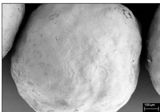
Figure IV.42. - SEM image of SEMP pellet; bar = 100 \mu\text{m} .
