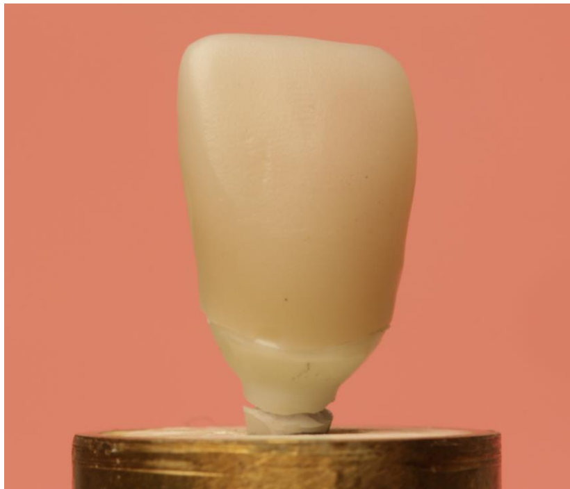
Figure 13: A specimen of group Zr broken at the abutment neck after quasi-static loading.
