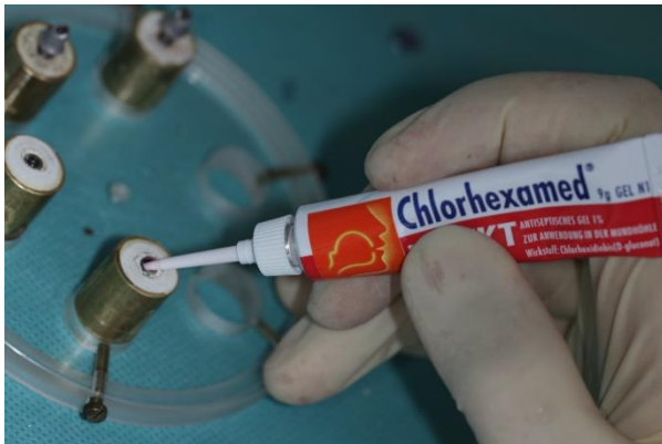
Figure 5: Applying antiseptic gel inside the internal connection of the implant before screwing the abutment finally to imitate the clinical situation.
