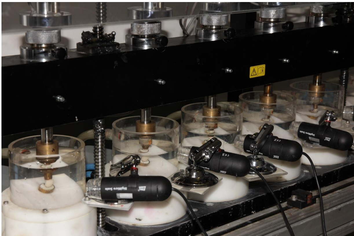
Figure 10: Test specimens during dynamic fatigue loading in the chewing simulator.
