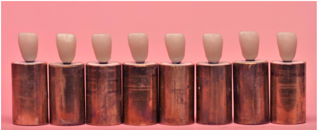
Figure 9: Eight complete specimens of group LaT after bonding and before starting the tests.
