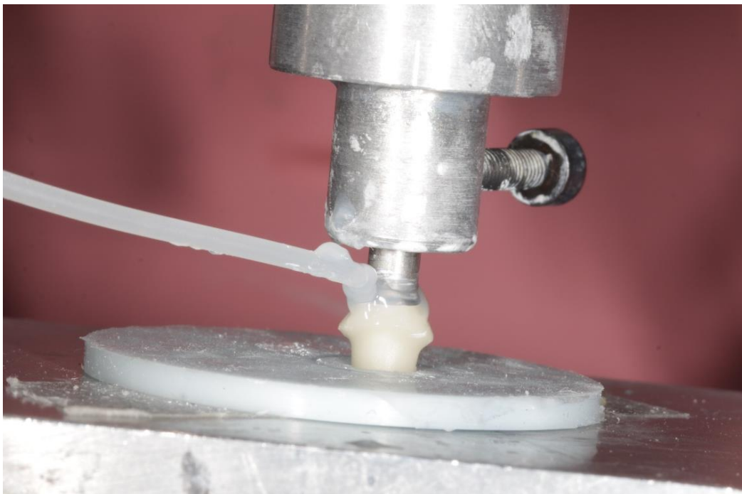
Figure 7: The ceramic suprastructure was bonded to the titanium insert under constant load of 750 grams to ensure uniform bonding technique for all specimens. As the load was applied, the excess cement was removed and glycerin gel was applied.
