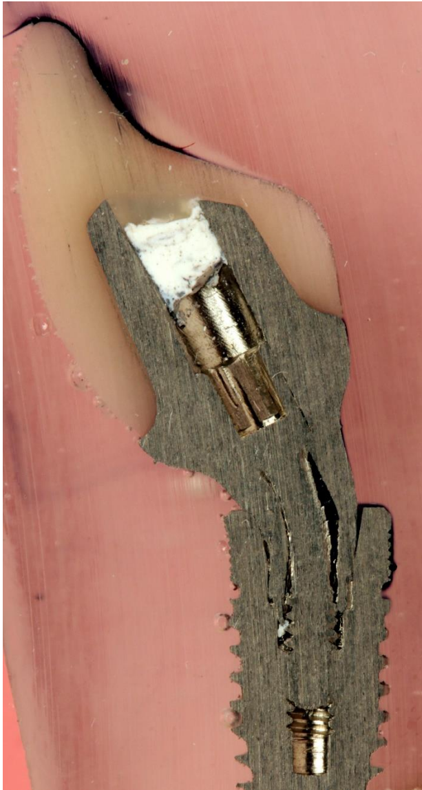
Figure 17: A sectioned specimen of group Ti, showing plastic deformation of the screw and the abutment without any fracture.
