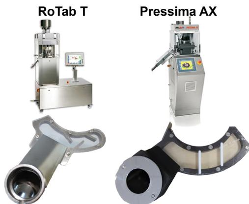
**Fig. 2.** Pictures of Rotab T (left) and Pressima AX (right). Top: Complete tablet press illustration. Bottom: Open feeder.
