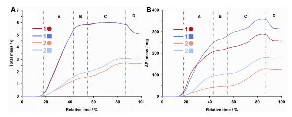
Fig. 9: (A) Total and (B) API mass filled into the die over time (confer for letters to text).
