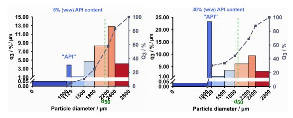
Fig. 2: Particle size distribution of the low (5% (w/w)) and high (30% (w/w)) API dose strength formulations.
