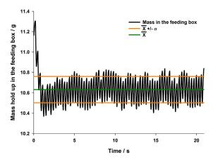
Fig. 5. Mass holdup obtained in the feeding box in the basic configuration over the complete discharge time (21 s). Lines indicate the mean and standard deviation.
