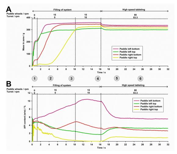
Fig. 2: (A) Mass and (B) API content during system filling and high speed tableting in four sections of the KIKUSUI force feeder (for the color code of the different sections confer to Fig. 3 & 5).
