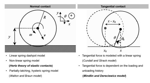
Fig. 5: Normal and tangential particle-wall contact schemes (particle illustration taken from [119]). The most popular models are listed.
