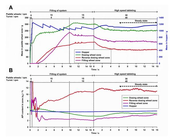
Fig. 4: Mass hold up (A) and API content (B) in different locations of the Fill-O-Matic over time during system filling (taken from our previous work [170] with permission from John Wiley and Sons) and high speed tableting.
