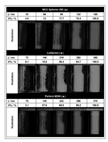
Figure 5. High-speed camera images at different time intervals during die filling of all materials with good flowing (one of the three measurements (Fig. 8)).
