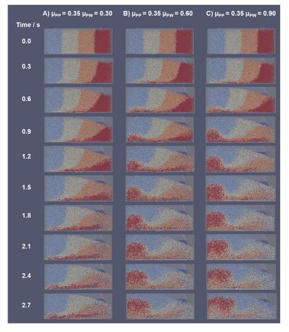
Fig. 15. Effect of particle-wall friction coefficient on particle rearrangement during the 10th die filling for different values of  $\mu_{PW}$ .
