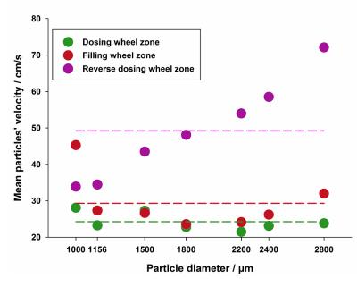
Fig. 8: Particles' velocity for the individual size fractions in the different paddle wheel zones during steady state. The dashed lines indicate the mean particles' velocity per zone.
