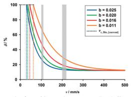
Figure 6. The influence of the DFI or decay rate constant (b) on die fill ratio ( $\delta$ ) at different die speeds (v) under constant  $\delta_{\min}$  (12%) and  $\delta_{\max}$  (178%) values (Equation (8)). The dotted line shows the corresponding  $v_{c, \text{ Die [current]}}$  at a given DFI (b). Grey zones (100 – 110 mm/s and 200 – 220 mm/s) are marked for comparison purpose, confer text.
