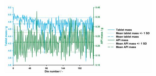
Fig. 5: Tablet mass and API content during 10 turret revolutions and 232 filled dies. The ranges between mean and mean  $\pm$  standard deviation are indicated in dashed and dotted lines, respectively.
