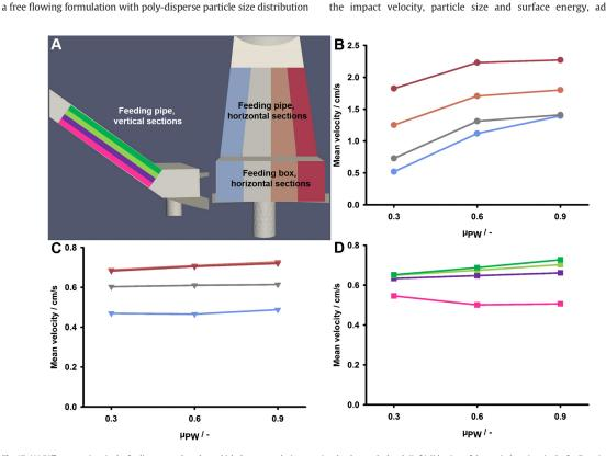
Fig. 17. (A) Different sections in the feeding system based on which the mean velocity over time has been calculated. (Left) Side view of the vertical sections in the feeding pipe, (right) front view of the vertical slices in the feeding pipe and feeding box. Quantitative comparison of the particles' mean velocities in the feeding system observed in (B) feeding box, horizontal sections, (C) feeding pipe, horizontal sections and (D) feeding pipe, vertical sections.
