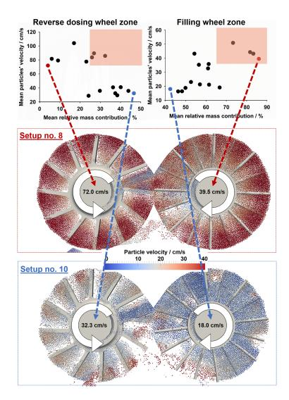
Fig. 7: Mean particles' velocity vs mean relative mass contribution (Fig. 6) for reverse dosing wheel (left) and filling wheel (right) zone (top) with exemplarily images for setup no. 8 and 10 (bottom, Tab. 1).
