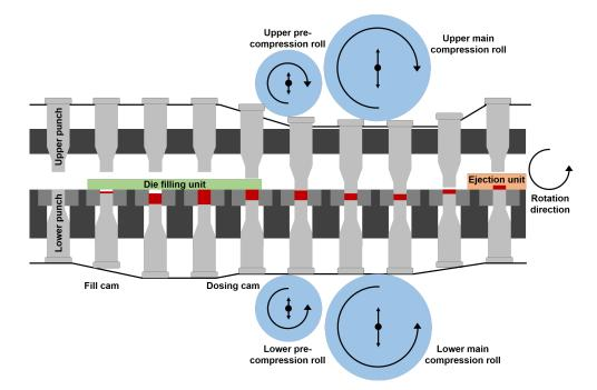
Fig. 1: Schematic illustration of a rotary tablet press.
