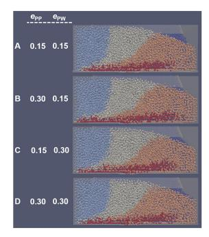
Fig. 19. Particle rearrangement in the feeding box during filling of the 10th die for different particle-particle ( $e_{PP}$ ) and particle-wall ( $e_{PW}$ ) restitution coefficients.
