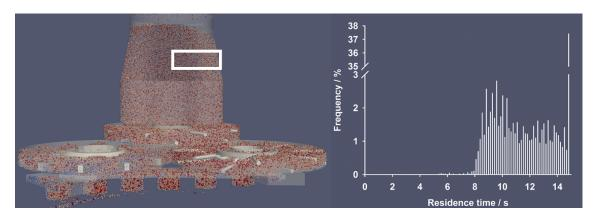
Fig. 11: Residence time distribution of all particles that were initially located in the top right hand half of the hopper (box, left).
