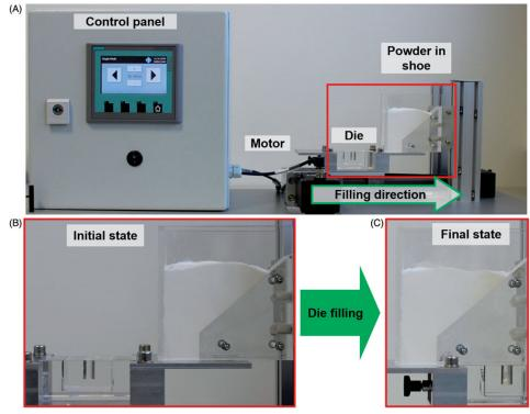
Figure 1. The new model die-filling setup including the complete setup (A) and the shoe and die before (B) and after (C) die filling.
