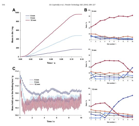
Fig. 8. (A) Mass collected in the die no. 10 with time for the die diameters of 6 mm, 9 mm, and 12 mm; (B) Distribution of the colored particles in the first 10 dies for 6 mm, 9 mm, and 12 mm die diameters as per their initial coloring within the feeding box; (C) Mass holdup in the feeding box for 6 mm, 9 mm, and 12 mm die diameters.
