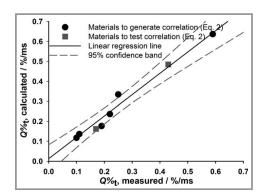
**Figure 10.** Verification of validity of Eq. (2) by comparing  $Q\%_t$  measured with  $Q\%_t$  calculated.
