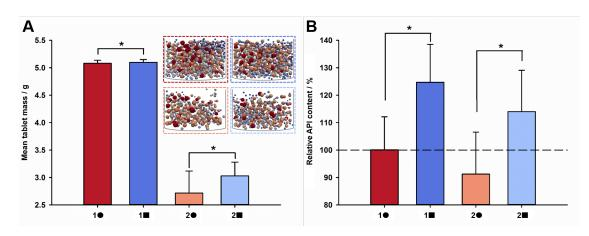
Fig. 8: (A) Mean tablet mass and (B) API content relative to label claim (\* significant difference in *t*-test). Exemplary screenshots of filled dies are given in Fig. 8A (confer to Fig. 3 for particle size legend).
