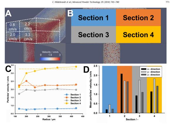
Fig. 4. (A) Mean particles' velocity in 4 sections of the feeding box that are defined in (B). (C) Mean particles' velocity per individual particle size in the 4 cross-sections of the feeding box and the complete box. The mean velocity over all sizes is given in dotted lines for the different locations, respectively. (D) Mean particles' velocity per x-, y-, and z-direction in the 4 cross-sections (confer Fig. 1 for directions).
