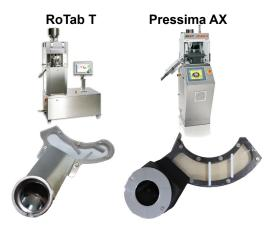
Fig. 2. Pictures of Rotab T (left) and Pressima AX (right). Top: Complete tablet press illustration. Bottom: Open feeder.
