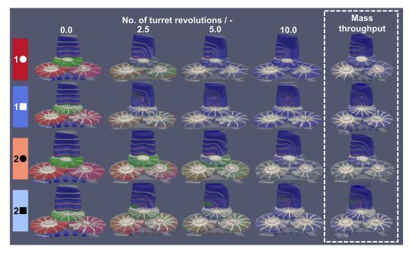
Fig. 10: Qualitative visualization of the traveling path of initially colored particles during high speed tableting and at the time point of same mass filled in the dies (quantitative in Fig. 11).
