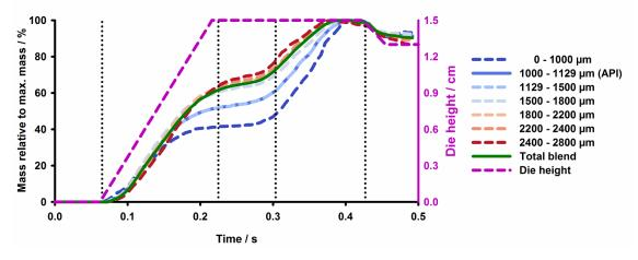
Fig. 6: Corresponding die height during filling of one die (pink). Relative mass to maximal mass (before dosing cam) that is obtained for each individual size fraction.
