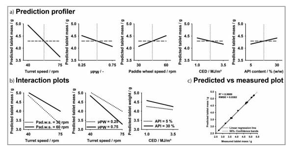
Figure 8. Prediction profiler (a), interaction plots (b), and predicted vs measured plot (c) of the tablet mass model.
