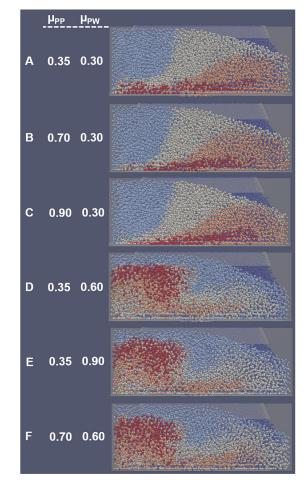
Fig. 14. Particle rearrangement in the feeding box during filling of the 10th die for different particle-particle ( $\mu_{PP}$ ) and particle-wall ( $\mu_{PW}$ ) friction coefficients.
