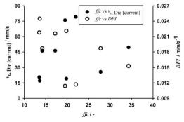
Figure 8. The (1) calculated critical die speed values ( $v_{c, Die [current]}$ , (2) DFI of different materials, and their corresponding measured ffc value.
