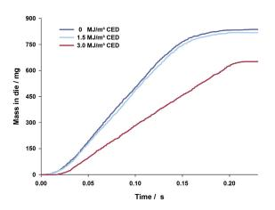
Fig. 9. Mass collected in die no. 10 with time for 0 MJ/m<sup>3</sup>, 1.5 MJ/m<sup>3</sup>, and 3.0 MJ/m<sup>3</sup> cohesion energy densities.
