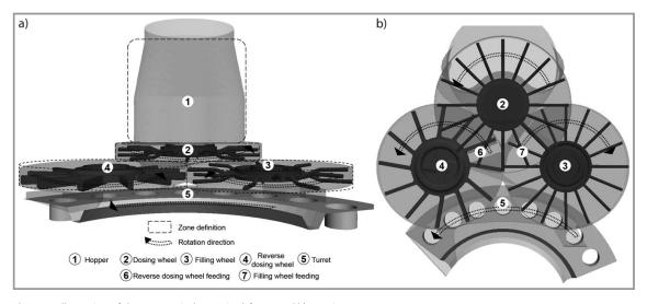
Figure 1. Illustration of the geometrical setup in a) front- and b) top view.
