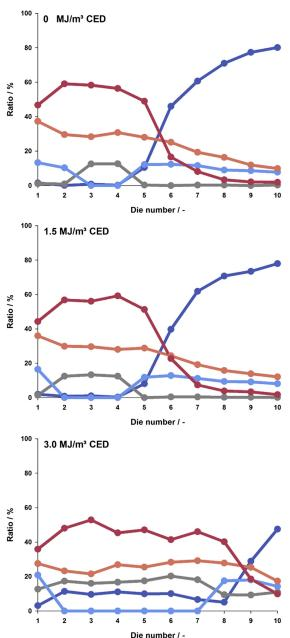
Fig. 11. Distribution of the colored particles in the first 10 dies for cohesion energy densities of 0 MJ/m<sup>3</sup>, 1.5 MJ/m<sup>3</sup>, and 3.0 MJ/m<sup>3</sup> as per their initial coloring within the feeding box.
