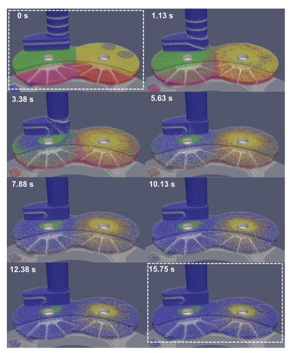
Fig. 5: Qualitative illustration of colored particles distribution at start of (t = 0 s) and during high speed tableting.
