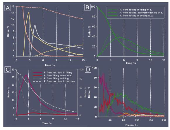
Fig. 10: Quantitative analysis of colored particles during discharge (for initial position of colors confer Fig. 9). (A) Ratio of colored particles in the hopper left hand half and right hand half (zones shown in Fig. 9, t = 0 s) and travel path of green (B) and red and pink (C) colored particles. (D) Colored particles in the filled dies.
