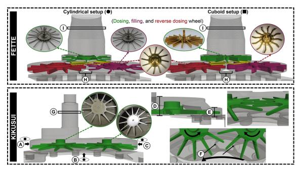
Fig. 1: FETTE (top, cylindrical and cuboid setup) and KIKUSUI (bottom) system illustrations (the images of the paddle wheels in KIKUSUI are shown in bottom view).
