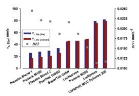
Figure 5. Calculated critical die speeds ( $v_{c, Die [Wu]}$  and  $v_{c, Die [current]}$ ) and comparison of DFI for different materials in the modified model die filling setup.
