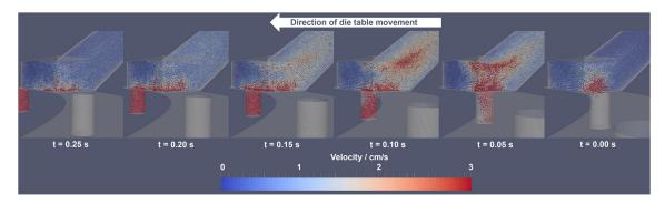
Fig. 3. Particle discharge from the feeding box into the 10th die. The die table moves with a constant rotational speed of 20 rpm in the *anti*-clockwise direction (indicated by the arrow). Particles are colored according to their velocity (red >3 cm/s and blue 0 cm/s). The interval between each image is 0.05 s. (For interpretation of the references to color in this figure legend, the reader is referred to the web version of this article.)
