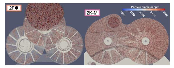
Fig. 7: Top view of force feeders during high speed tableting for FETTE 2F● and KIKUSUI 2K-M setups.
