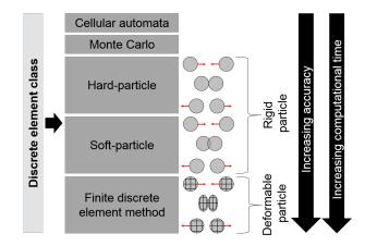
Fig. 2: Overview of different discrete element classes
