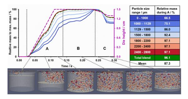
Fig. 4: Mass filled into the die relative to maximal mass per particle size fraction underneath (A) RHSP, (B) LHSP, and (C) dosing cam. Table: Mass relative to max. mass filled from RHSP into the die for different particle size fractions. Bottom: Screenshots of die during filling where particles are colored according to their size (for scale refer to Fig. 3).
