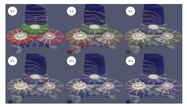
Fig. 9: Tracking of particles, colored by their initial position during high speed tableting at intervals of 3 s.
