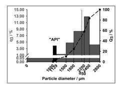
**Figure 2.** Particle size distribution consisting of seven different sizes, out of which one particle size reflects API particles and the remaining are excipient particles.
