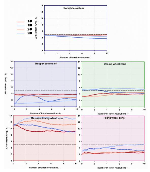
Fig. 13: API content during high speed tableting in different locations of the system (normalized to no. of turret revolutions for condition 1 and 2).
