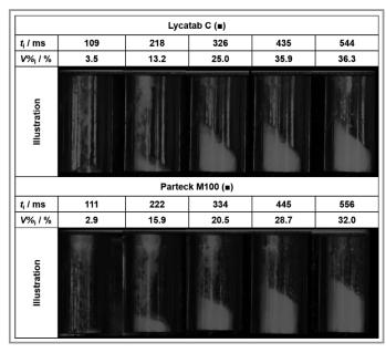
Figure 7. High-speed camera images at different time intervals during die filling of all materials with bad flowing (one of the three measurements (Fig. 8)).
