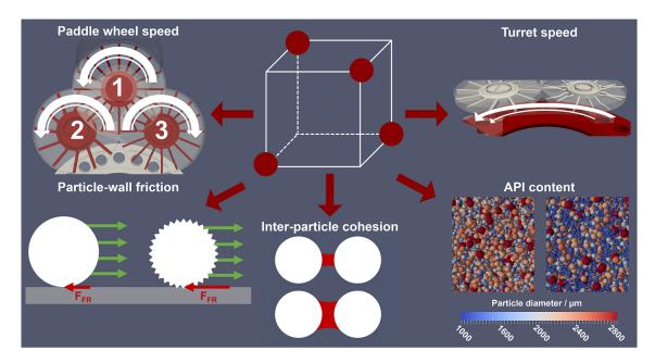
Fig. 1: Schematic illustration of the screening design and the included factors.
