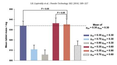
Fig. 12. Mean tablet mass over 70 filled dies for different particle-particle ( $\mu_{PP}$ ) and particle-wall ( $\mu_{PW}$ ) friction coefficients. Statistical analysis: One way ANOVA and Bonferroni's post *t*-test ( $\alpha = 0.05$ ). Pairs having *P* values >0.05 are indicated.
