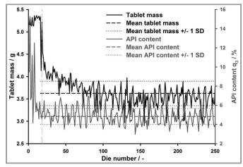
Figure 7. Tablet mass and API content during 10 turret rotations and 240 filled dies.
