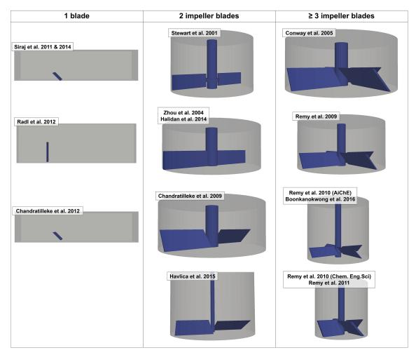
Fig. 1: Systematic illustration (reconstructed from original) of the different impeller blade studies ordered by their number of impeller blades (different scales).
