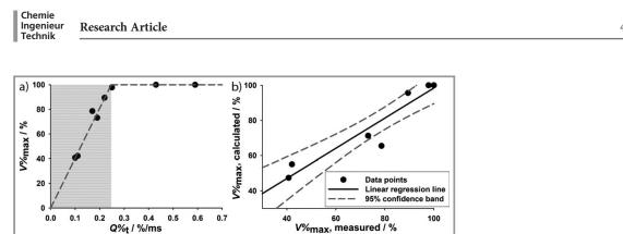
**Figure 11.** a)  $V\%_{max}$  vs  $Q\%_t$  data points. The gray-line inked zone highlights data points with  $V\%_{max} < 100 \%$ . Dashed lines are linear regression lines for  $V\%_{max} < 100 \%$  and  $V\%_{max} \ge 100 \%$ , respectively. b)  $V\%_{max}$  calculated via  $Q\%_t$  calculated (obtained through particle size information (Eq. (2) and Eq. (3)) vs  $V\%_{max}$  measured.
