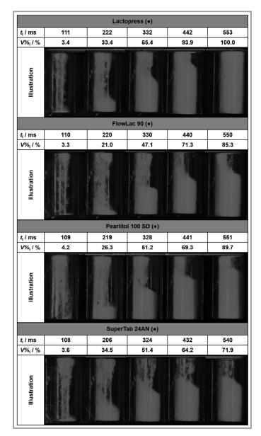
**Figure 6.** High-speed camera images at different time intervals during die filling of all materials with intermediate flowing (one of the three measurements (Fig. 8)).
