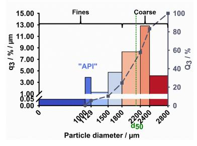
Fig. 3: Particle size distribution of the simulated DC formulation.
