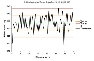
Fig. 4. Tablet mass obtained in the basic configuration for 70 filled dies. Lines indicate the mean, and one and twofold standard deviations.
