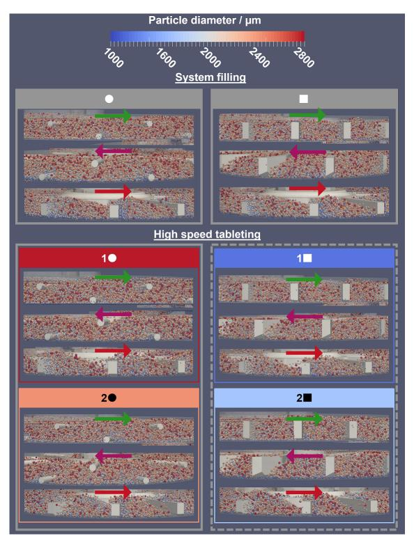
Fig. 7: Particle size distribution during system filling and at the end of high speed tableting. The arrows (color code refers to paddle wheels Fig. 2) indicate the rotation direction.
