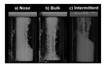
Figure 1. Examples for a) nose, b) bulk, and c) intermittent flow.
