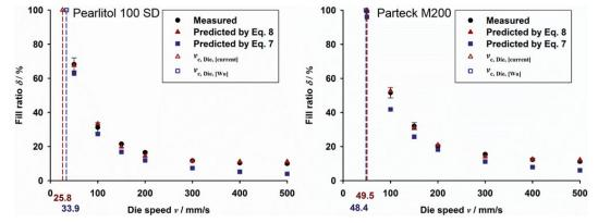
Figure 4. Comparison of fill ratio prediction by power law relationship, proposed by Wu et al. (Equation (7)), and exponential decay rate (Equation (8)). The dotted lines indicate the  $v_{c, Die [Wu]}$  (by Equation (7)) and  $v_{c, Die [current]}$  (by Equation (8)).
