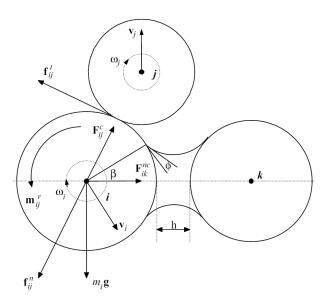
Fig. 3: Forces acting on particle i from contacting particle j and non-contacting particle k via capillary force are schematically shown. Illustration taken from [23].
