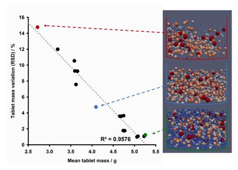
Fig. 4: Tablet mass variation vs tablet mass; for setup nos. 10 (top, red), 14 (middle, blue), and 3 (bottom, green) exemplary dies are shown.
