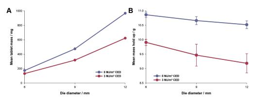
Fig. 21. Effect of the combination of different die diameters (6 mm, 9 mm, and 12 mm) with CED values (0 and 3.0 MJ/m<sup>3</sup>) on (A) mean tablet mass, and (B) mass holdup in the feeding box.
