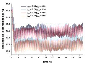
Fig. 18. Variation in shoe mass holdup under different coefficients of friction.
