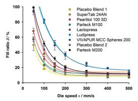
Figure 3. The effect of die speed (v) on the die fill ratio ( $\delta$ ) for different pharmaceutical powders. Lines are generated by applying Equation (8).
