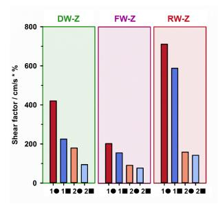
Fig. 15: Shear factor in the different paddle wheel zones according to Eq. 1.
