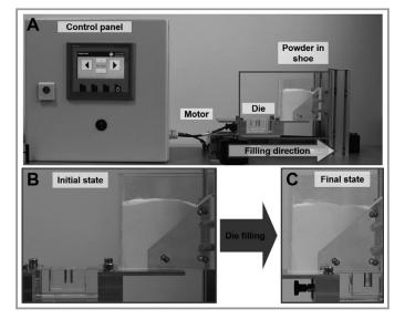
Figure 2. The new model die filling system including the complete setup (top) and the shoe and die before (bottom left) and after (bottom right) die filling [11].
