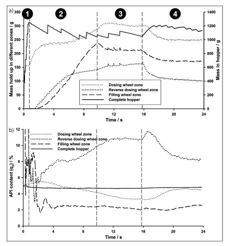
Figure 4. Mass holdup (a) and API content (b) in different locations of Fill-O-Matic over time. Same time intervals as listed in Tab. 2 are indicated.
