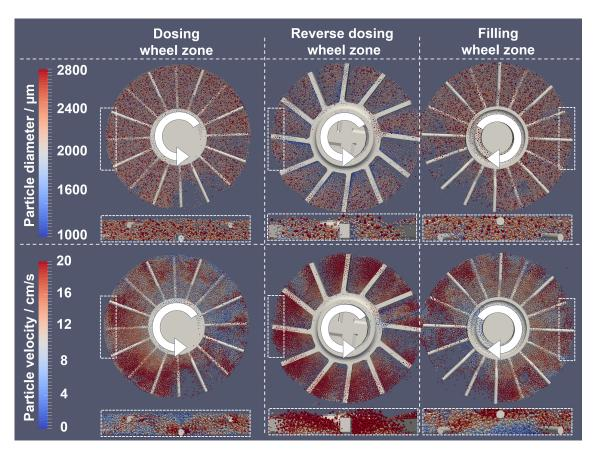
Fig. 7: Top and side view of the three individual paddle wheel zones with particles colored according to their size (top) and their velocity (bottom).
