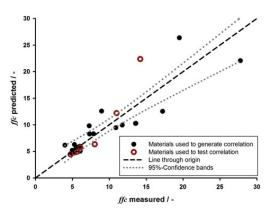
Figure 2. The *ffc* measured versus *ffc* predicted for 28 materials. The materials used in generating the correlation (Equation (6)) are indicated in black, filled circles, whereas the materials used for correlation validation are shown in red, unfilled circles.
