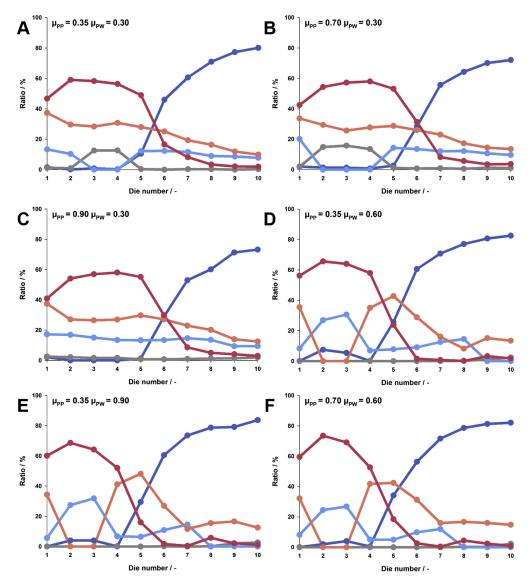
Fig. 16. Distribution of the colored particles in the first 10 dies under different friction coefficients ( $\mu_{PP}$  and  $\mu_{PW}$ ) as per their initial coloring within the feeding box.
