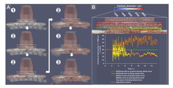
Fig. 3: Illustration of the system during filling (A), numbers correspond to steps in Tab. 2). (B) Content of particles ≤ 1800 µm in three horizontal zones of the dosing wheel zone and in the refilling regions of the reverse dosing wheel zone and the filling wheel zone during system filling (A).
