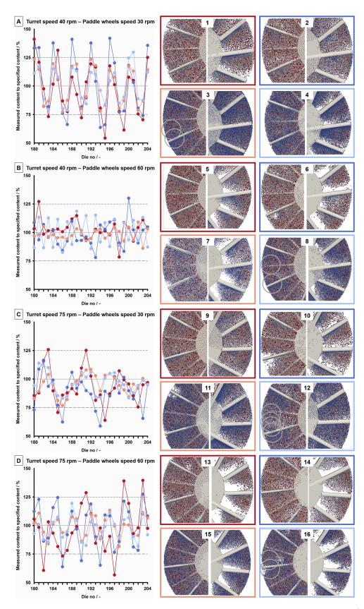
Fig. 5: Relative API content over tableting time and instantaneous images of the bottom of the filling wheel (left) and reverse dosing (right) wheel zone (particles are colored by their size, confer as legend to Fig. 1 & 2):
