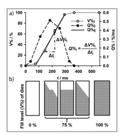
**Figure 4.** a) Volume fill ratio  $(V\%_i)$ , local volume flow rates  $(Q\%_i)$  and total volume flow rate  $(Q\%_i)$  vs time for Parteck M200. b) Schematic illustration of different volume fill ratios of dies.
