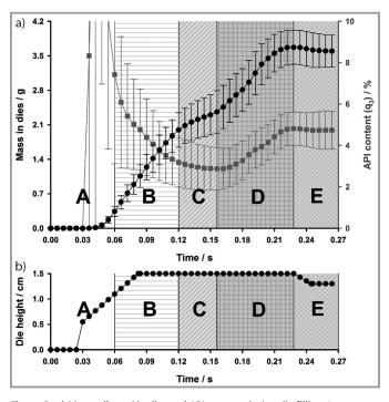
Figure 6. a) Mass collected in dies and API content during die filling. Letters and sections indicate corresponding positions within the Fill-O-Matic as shown in Fig. 5. b) Die height as it changes over filling time.
