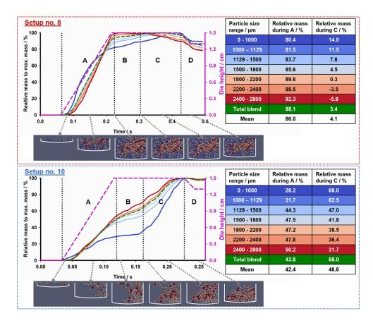
Fig. 6: Relative mass to maximal mass for individual particle size fractions and die height over filling of one die are shown. The die is located under the filling wheel ('A'), inter-wheel ('B'), reverse dosing wheel ('C'), and dosing cam ('D') zone.
