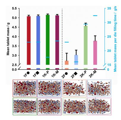
Fig. 6: Mean tablet mass (left y-axis) and mean tablet mass per die filling time (right y-axis) for the different setups. Bottom: Exemplary filled dies for all setups (confer for color code to graph legend). Particles are colored by their size (for scale refer to Fig. 3).
