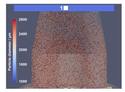
Fig. 14: Particle size distribution in the feeding hopper at the end of high speed tableting for setup 1
