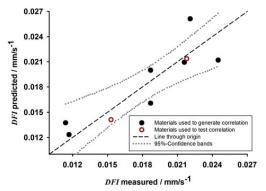
Figure 7. The comparison of measured and predicted (by Equation (9)) values of DFI. The materials used in generating the correlation (Equation (9)) are indicated in black, filled circles whereas the materials used for correlation validation are shown in red, unfilled circles.
