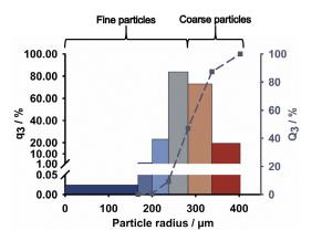
Fig. 2. Particle size distribution of the VIVAPUR MCC Spheres determined by laser diffraction. The bar colors of the individual sizes are subsequently used in illustrations.
