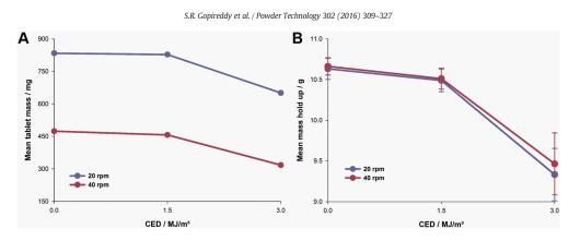
Fig. 20. Effect of the combination of different die table speeds (20 and 40 rpm) with CED values (0-3.0 MJ/m<sup>3</sup>) on (A) mean tablet mass, and (B) mass holdup in the feeding box.
