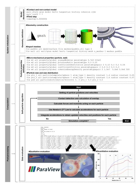
Fig. 4: Example flowsheet for DEM simulation including pre-processing (input file contains only most important commands necessary in LIGGGHTS [116]), computation via soft-particle algorithm (adapted from [20]), and postprocessing.
