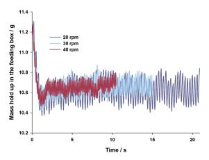
Fig. 7. Mass holdup in the feeding box for 20 rpm, 30 rpm, and 40 rpm die table speeds.
