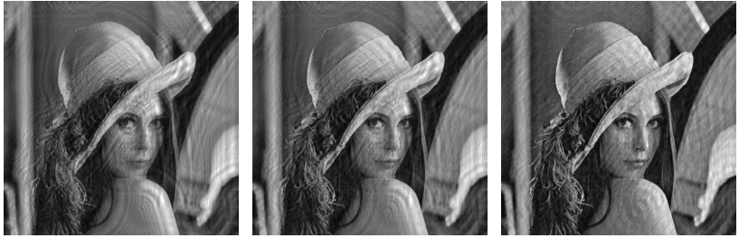
(a) PSNR 26dB with 3 iterations of WFC-HAAR (b) PSNR 28dB with 5 iterations of WFC-HAAR (c) PSNR 31dB with 15 iterations of WFC-HAAR
