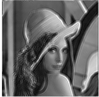
(b) Defocus with maximum wavefront deformation of -25\lambda
