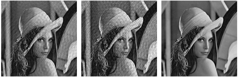
(d) PSNR 33dB with 25 iterations of WFC-HAAR (e) PSNR 40dB with 100 iterations of WFC-HAAR (f) PSNR 47dB with 500 iterations of WFC-HAAR
