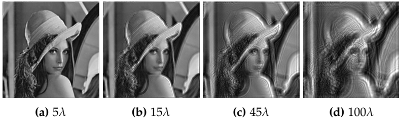
Figure 4.1. Defocus of increasing strength applied on an image, measured in maximum wavefront modulation in wavelengths.
