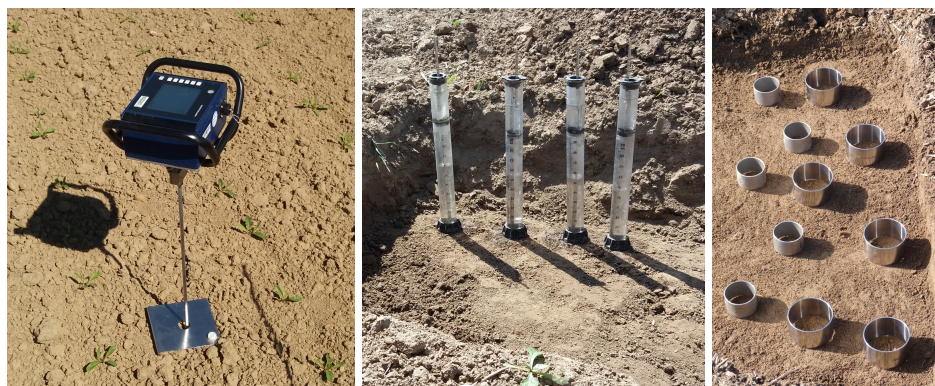
Figure 3.4: Field equipment: Penetrologer (left), mini-disc infiltrimeter (middle) and core samples (right).
