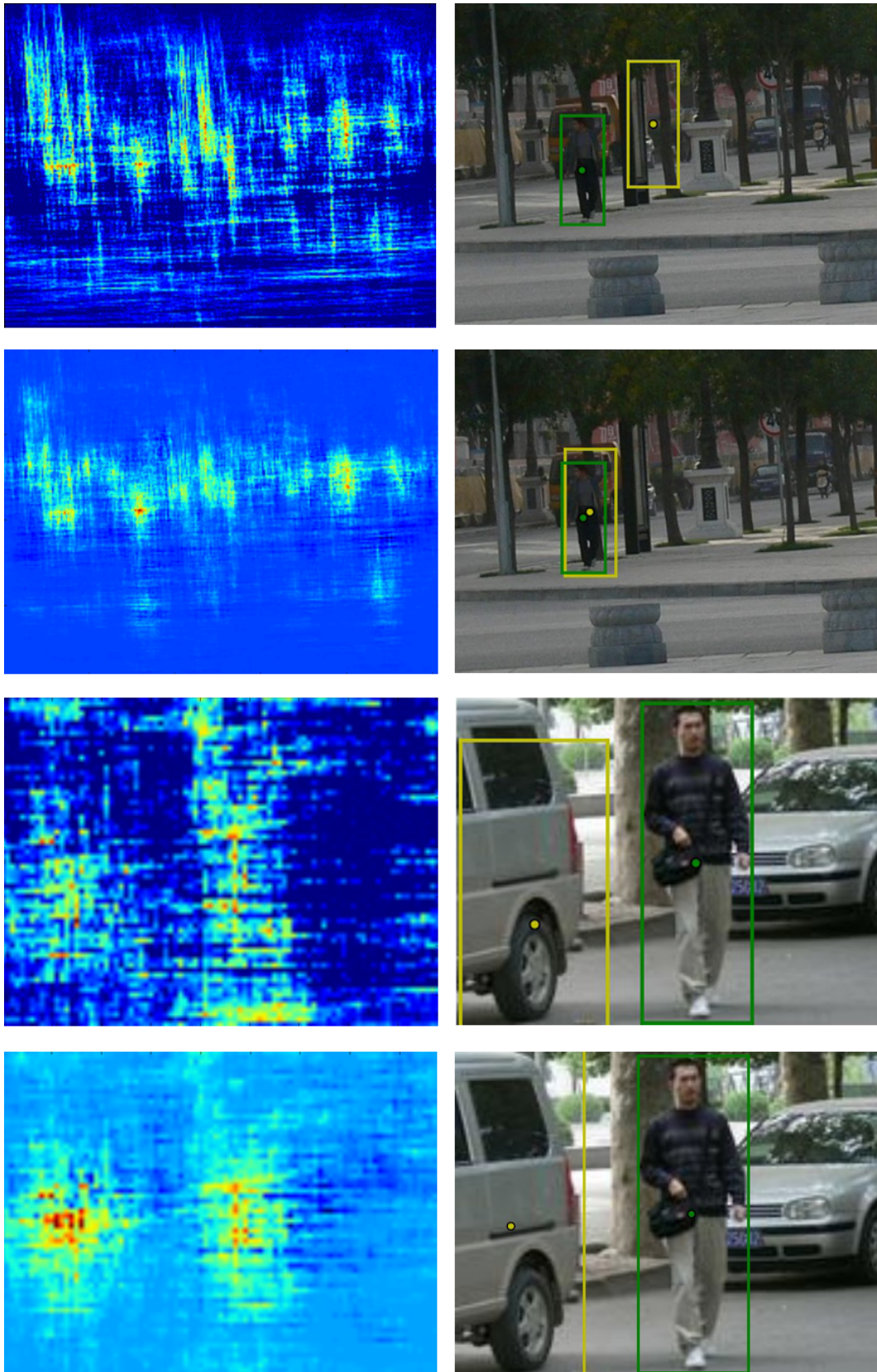
FIGURE 4.8: Example Hough spaces and corresponding detection results on the IAIR Pedestrian Subset. Odd rows: DGHT only, even rows: DGHT+SCM. (Left) Hough space (Right) Detection result; yellow: prediction, green: ground truth annotation. (Best viewed in color.)
