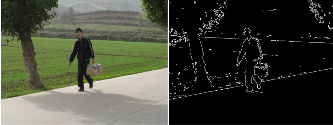
FIGURE 2.3: (Left) Input image. (Right) Canny edge image.
