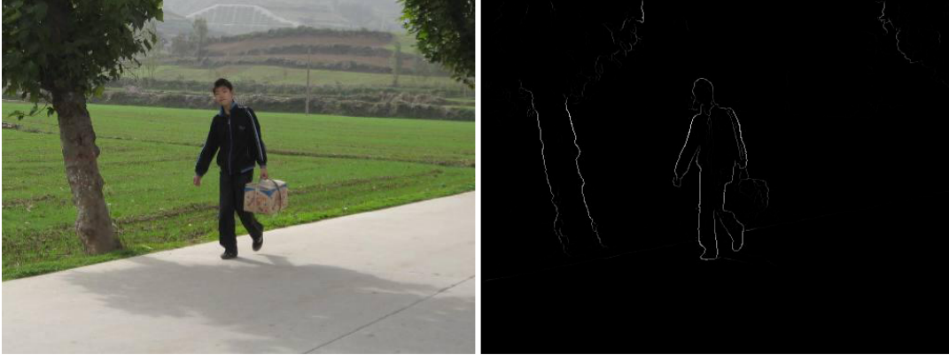
FIGURE 2.4: (Left) Input image. (Right) Structured edge image trained on pedestrian contours.
