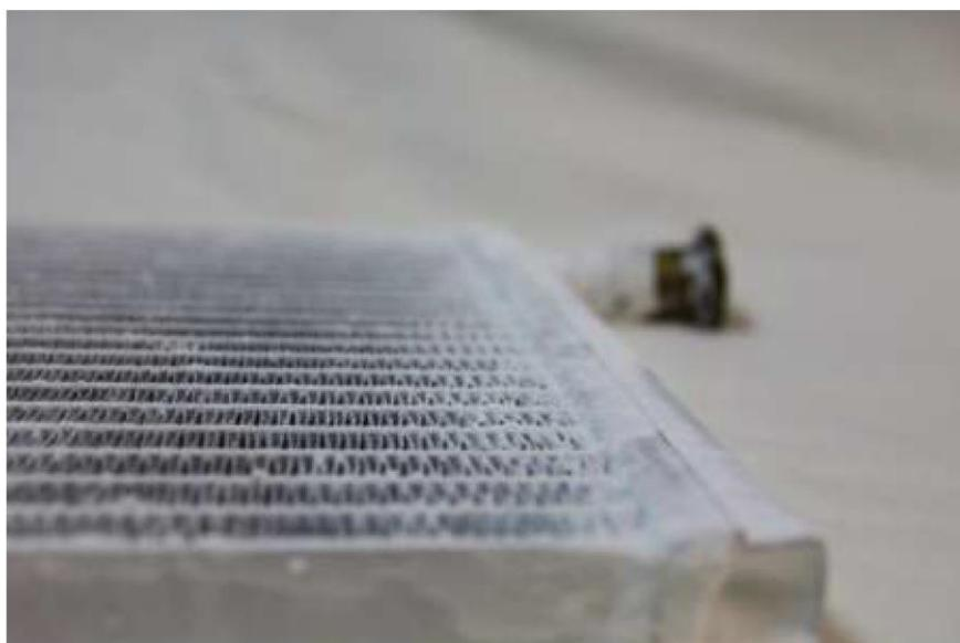
**Figure S20.** Picture of coated heat exchanger.
