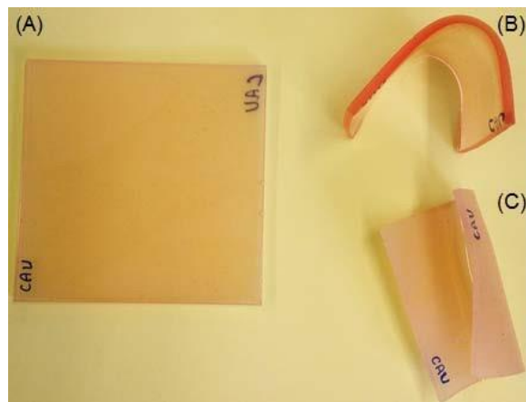
Fig. 3 Different shapes of the PTU/spiropyran under temperature controlled conditions. (A) Corresponds to the original shape of PTU/spiropyran, (B) and (C) are folded and twisted shape of PTU/spiropyran respectively
