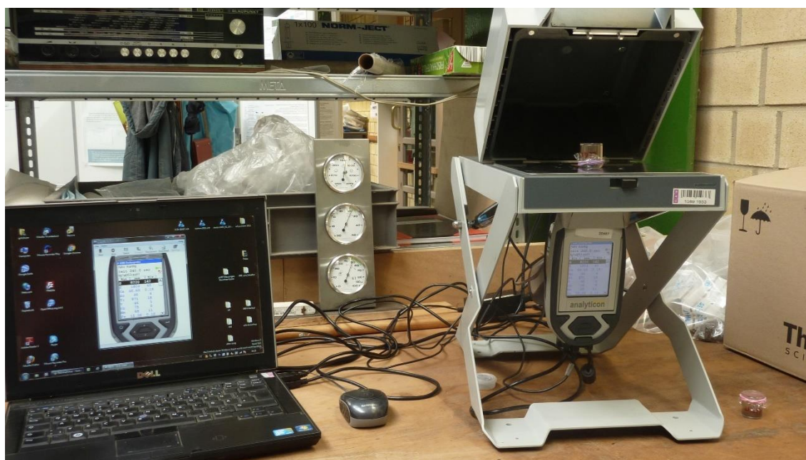
Figure 3: The pXRF with connected sampling chamber.
