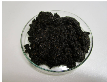
Figure 6.3: A sample of a high grade oil sand used in this study.
