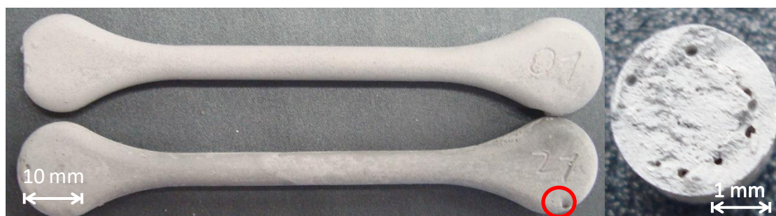
Figure 5-5 Injection moulding defects of samples with isotactic PP backbone polymer. Left top sample minor defects of non-recycled feedstock, bottom sample of recycled feedstock with demixing (different coloured areas) and improper filling (red circle). Right picture displays air entrapments inside the part.
