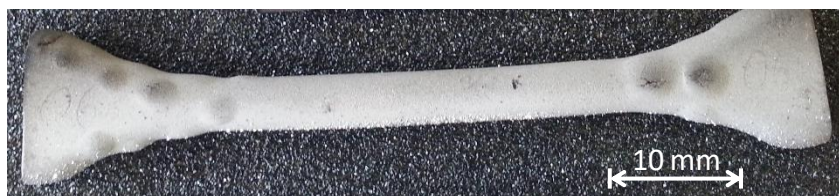
Figure 5-26 Blister formation on PE-EVA MIM samples after sintering.
