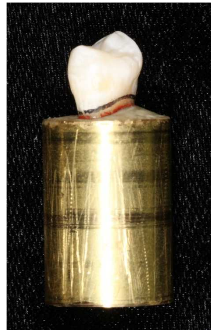
Figure 3: Embedment in auto-polymerizing polyester resin.
