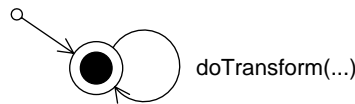
Figure 8.11: Finite state automaton defining the provided protocol of the Presentation Format Generators component
