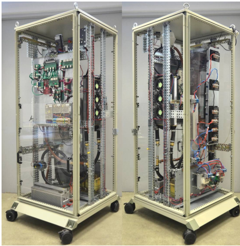
Figure 9: Test bench for Power-Stack at low power (up to 20 kW).
