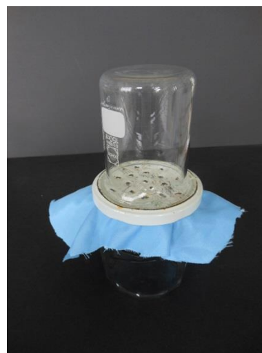
Figure 49: Setup for testing steam permeability of a textile
