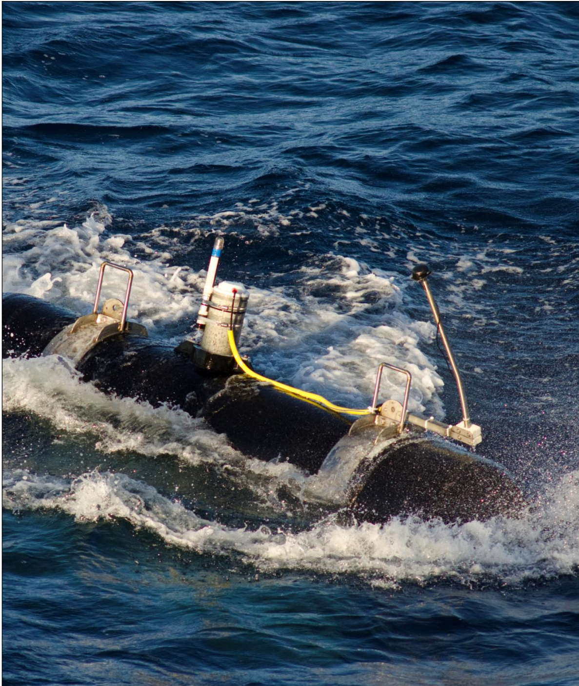
Portside paravane of the high-resolution P-Cable seismic system offshore New Zealand
