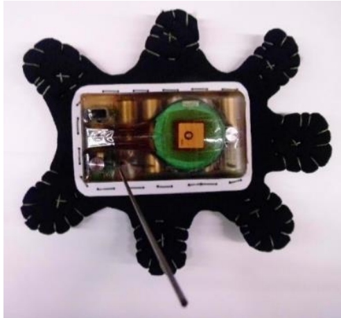
Fig. S1: Tags were attached to a rectangular neoprene base with seven €2-sized small feet at its edges. Only these feet were glued to the fur to break up the glue patch. The tags would thus fall off during the next moult, if not before.
