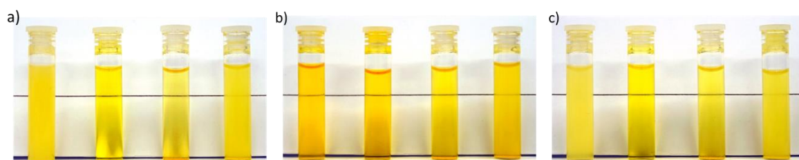
Figure 6.6: Reversible solubility switching of the different macrocycles in water at a concentration of 500 \mu\text{g/mL} : (a) trans -rich samples; (b) after irradiation with 365 nm for 10 min; (c) after irradiation with 520 nm for 10 min; from left to right: \alpha -mannoside 27 , \alpha -glucoside 28 , \beta -glucoside 29 , \beta -galactoside 30 .
