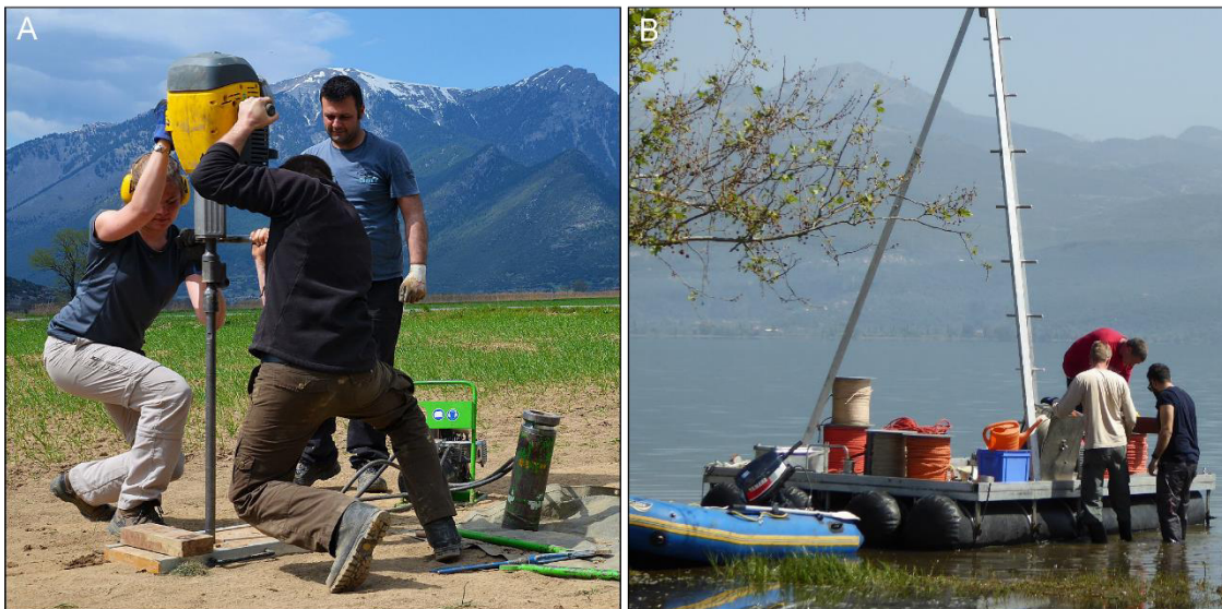
Figure 4: Coring campaigns. (a) March 2017, coring palaeolake Pheneos with a piston corer (photo: I. Unkel). (b) April 2018, installation of the coring platform at Lake Trichonida (photo: J. Seguin).
