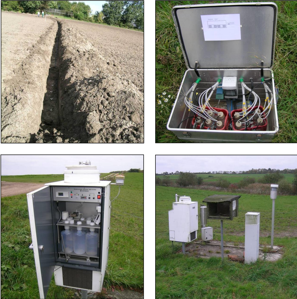
Figure 5: Devices used in the intensive monitoring: Installation of leachate samplers (upper left, picture: D. Elsner), leachate collection box (upper right), wet-only collector for deposition (lower left), deposition measurement station (lower right), pictures except upper left: R. Nerger, 2007-2008
