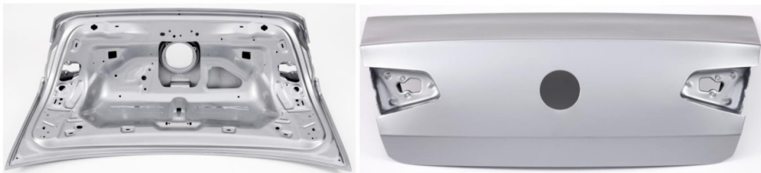
Figure 12. Tailgate for Volkswagen Passat utilizing a twin-roll-cast (TRC) Mg-Zn-Ca-Zr sheet [277] (pictures offered by Volkswagen. Copyright accessed).
