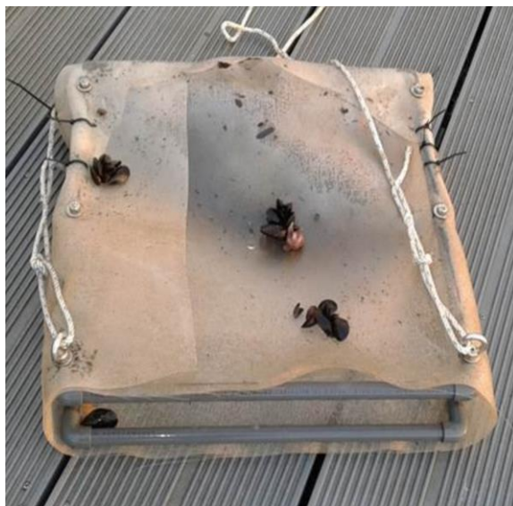
Figure S2. Trap design for catching crabs, consisting of 50 \times 50 \times 20 cm PVC pipes covered entirely with a 1 mm mesh, allowing mussel predators to enter on both sides. The traps were regularly filled with crushed Mytilus edulis mussels.
