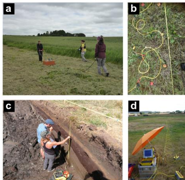
Figure 3: picture from the field during the different geophysical campaigns. a) GPR measurements done pulling the 200 MHz antenna on the ground in 2017; b) Geophones on the ground during the seismic
