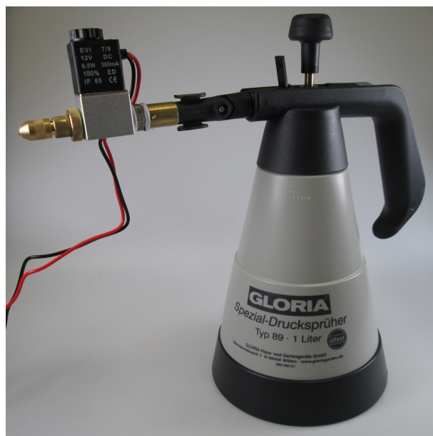
Figure 2.9: Gloria Type 89 pressure sprayer connected with solenoid valve.
