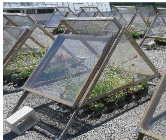
Figure III.S2: Technical drawing of UV cabinets equipped with plastic filter sheets (blue) and photo of the experimental setting in the New Zealand common garden
