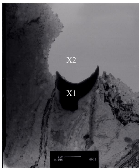
Fig. S1. TEM image of the intermetallic particle after twin-jet electropolishing with 1.5% perchloric acid solution
