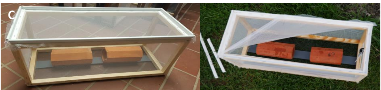
Figure 4.2: Enclosure type C: 60 x 25 x 25 cm (L x W x H), wooden framework, sides covered with gauze (1.5 mm mesh size), removable top cover by means of built-in clip system, 2 clay pipes placed inside, construction placed at a depth of 1.30 m.
