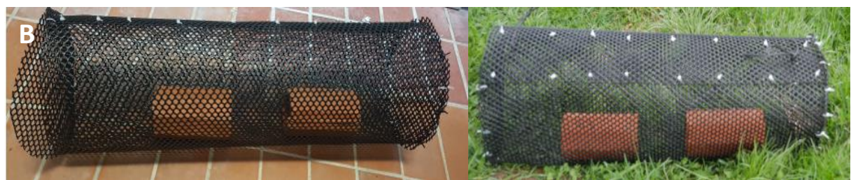
Figure 4.3: Enclosure type B: 70 cm side length and 22 cm diameter, tubular enclosure made of wire fence (8 mm mesh size), 2 clay pipes placed inside, construction placed at a depth of 1.30 m.
