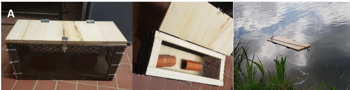
Figure 4.1: Enclosure type A: 60 x 25 x 25 cm (L x W x H), wooden top and bottom (Paulownia wood, 1.8 cm thickness), hinged top cover, sides covered with wire fence (8 mm mesh size), 2 clay pipes placed inside, construction balanced with weights to float just below the water surface.
