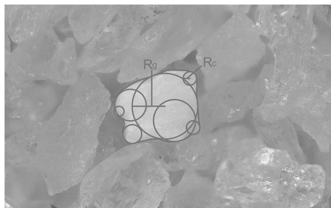
(c) Zoom-in of the box in subfigure (b). Measuring R_g and R_{ci} to determine R_W
