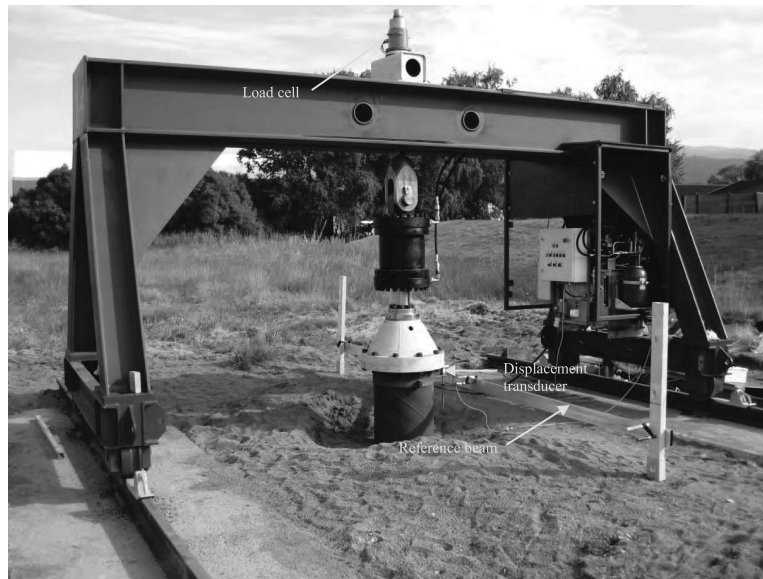
Figure 2.2: Loading system setup used at test sites [Karlsruud et al., 2014]
