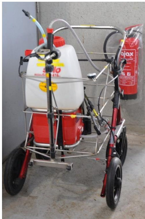
Figure 1 Application system with the automatic backpack sprayer in a newly built metal cage and a front extension for the spray bar and the two nozzles.
