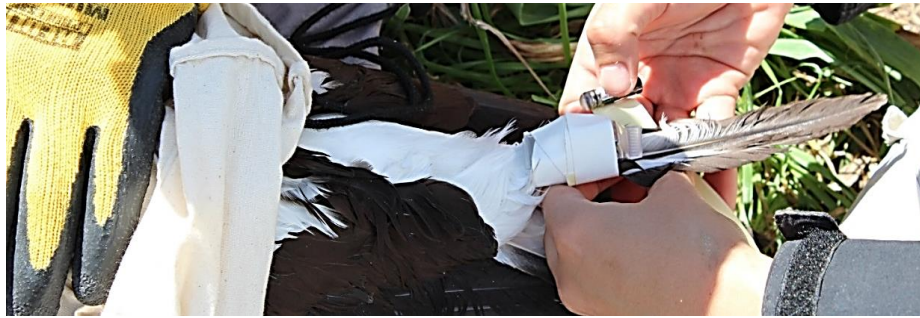
Figure 1.5. Attachment of GPS and TDR devices to the central rectrix feathers of a masked booby using waterproof tape.
