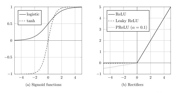
Figure 2.4: Frequently used activation functions for DNNs. Sigmoid functions (a) have been used for a long time in ML. Today, rectifiers (b) are more commonly used for training neural networks. The variable  $\alpha$  in the PReLU activation function is trained like the other network variables. The value of  $\alpha = 0.1$  was chosen freely for this figure. Note that there are more well known activation functions, these are just the ones that are important for this work.
