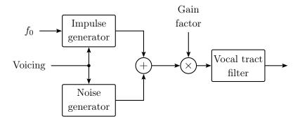
Figure 3.6: Source-filter model of speech production. Generally, for voiced speech, the impulse generator is used and for unvoiced speech, noise is generated. The combination of both is also possible as both generators can produce signals at arbitrary levels independently of each other. The vocal tract is modeled as digital filter.
