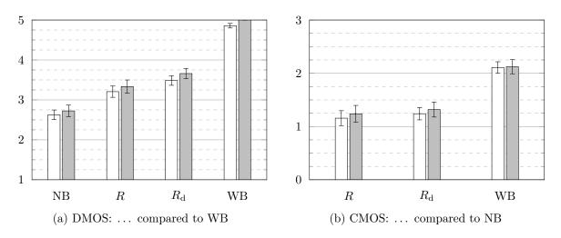
Figure 7.5: Mean speech quality ratings (bars) and 95% confidence intervals  $c_{95}$  (error plots) of the DMOS test (a) and the CMOS test (b). The results are shown for all listeners (white) and selected listeners (gray). The y-axis in (b) is just shown for positive values as NB was rated worse than all compared categories.
