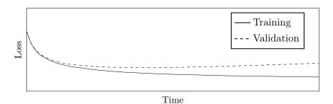
Figure 2.3: The training loss (solid line) and the validation loss (dashed line) are plotted for the duration of a training process. It can be seen that the validation error stops to decrease at a certain point and increases again. This is a clear signal for overfitting in the training process.
