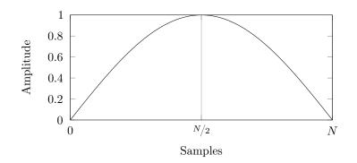
Figure 3.10: Analysis window  $w_{\text{ana}}(n)$  that is used in the filterbank. The synthesis window  $w_{\text{syn}}(n)$  is identical. It is a square-root Hann window that leads to perfect reconstruction with an overlap of 50%.
