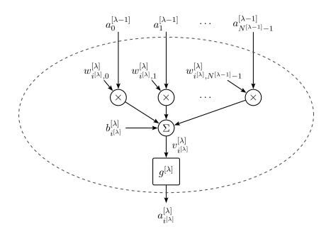
Figure 2.2: Artificial neuron at index  $i^{[\lambda]}$  in layer  $\lambda$  of an MLP for  $\lambda > 0$ . In the input layer ( $\lambda = 0$ ), the inputs are just forwarded to the next layer. Note that there are exceptions in which the activation function  $g^{[\lambda]}$  depends on the whole vector  $\mathbf{v}^{[\lambda]}$ .
