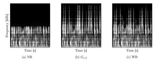
Figure 7.8: NB, ABE, and WB spectra for the left channel of a binaural signal that was used in the listening test.
