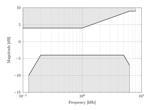
Figure 3.9: Attenuation limits for the hands-free sending path of cellphones, adapted from ITU-T rec. P.341 [ITU11a].
