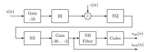
Figure 7.1: Block diagram of the training data generation process for a DNN that predicts the WB spectral envelope from features that are based on the NB signal. z(n) is a background noise signal that is added to a processed version of the speech signal s(n). IR denotes a convolution with an impulse response, EQ denotes a convolution with an equalizer filter, NS represents a noise suppression algorithm, and NB denotes a convolution with a narrowband filter. The gains are given in dBFS.
