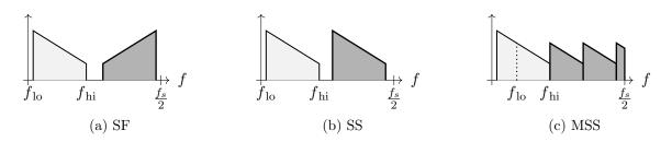
Figure 4.3: Schematic spectra for the three excitation extension methods: SF (a), SS (b), and MSS (c). The dark parts represent the generated extension spectrum, the light parts represent the original NB spectrum.
