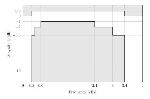
Figure 3.8: Attenuation limits for circuits with 4-kHz channel equipment, adapted from ITU-T rec. G.120 [ITU98].
