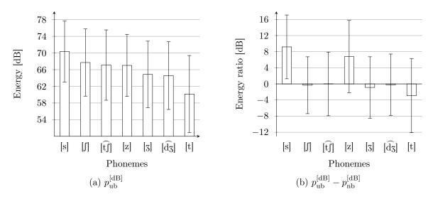
Figure 3.3: Comparison of the mean energy of phonemes in the TIMIT dataset in dB (the speech files were read as 16-bit integer values). Just the seven phonemes with the highest energy in the UB (above 3.4 kHz) are shown. The comparison results are shown for the UB energy (a) and for the ratio between the UB energy and the NB energy between 0.3 and 3.4 kHz (b). The error bars represent the standard deviation towards lower and higher values.
