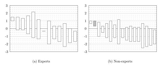
Figure 7.10: Listener-based evaluation of  $G_{c,d}$  compared to NB and WB for expert (a) and non-expert (b) listeners. Each bar represents one listener with the NB-to- $G_{c,d}$  rating as lower end and the WB-to- $G_{c,d}$  rating as upper end of the bar. Only for the single gray bar, the limits are swapped because in comparison with  $G_{c,d}$ , the listener rated NB better than WB. The horizontal line at a value of zero represents the quality of  $G_{c,d}$ .
