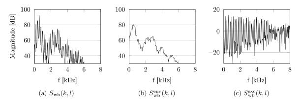
Figure 4.2: Spectrum of the vowel [æ] in the word 'favor'. The original WB spectrum  $S_{wb}(k,l)$  (a) is decomposed into the spectral envelope  $S_{wb}^{env}(k,l)$  (b) and the excitation spectrum  $S_{wb}^{exc}(k,l)$  (c).
