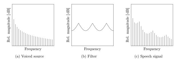
Figure 3.7: Schematic example of the source-filter model of speech production for a voiced speech sound. The voiced sound source (a) is filtered with the characteristics of the vocal tract (b) and produces the speech signal (c).
