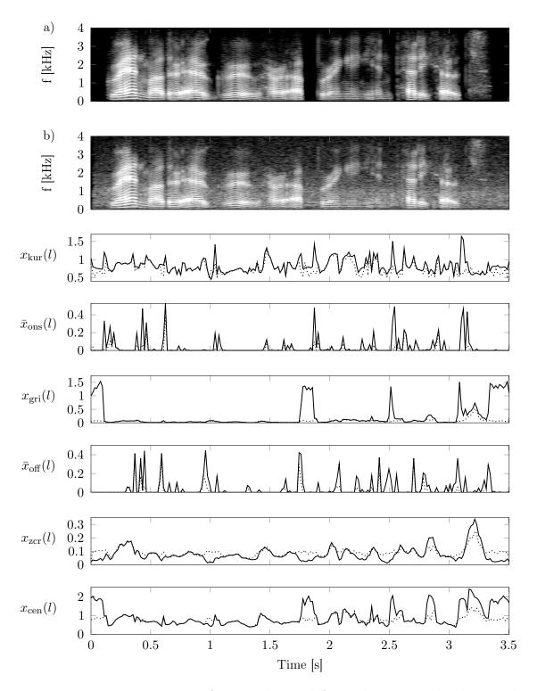
Figure 6.1: NB spectrogram of a speech signal from the TIMIT database with a comparison of several features. The clean NB spectrogram is depicted in (a). A noisy version, in which driving noise is added with an SNR of 10 dB, is shown in (b). The following graphs show the local kurtosis, the onset feature, the gradient index, the offset feature, the zero crossing rate and the centroid. The dotted graphs refer to the noisy signal while the solid graphs represent the clean speech.
