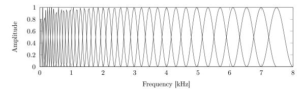
Figure 3.11: Superposition of all filters of the mel filterbank that was used in this thesis. Each filter is formed by a single sine wave instead of a rectangle, which is often done in literature, for smoother transitions. The filters are normalized to a sum of 1 for the conversion to a mel spectrum. For the conversion back to the FD, the filters are not normalized, as displayed in the figure.
