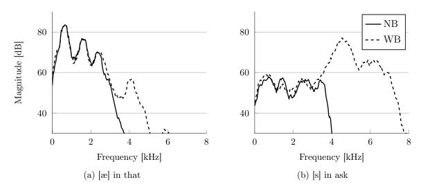
Figure 4.4: WB (dashed) and NB (solid) short-term spectral envelopes of the phoneme [æ] in the word 'that' (a) and the phoneme [s] in the word 'ask' (b). The spectra were extracted from recordings that were made with a network simulator and a cellphone. The NB signal was recorded after the simulated transmission with the AMR codec at 12.2 kbps and the WB signal after the AMR-WB codec at 12.65 kbps.
