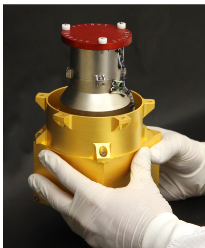
Figure 5: A photo of the RAD sensor head before it was mounted on the MSL spacecraft. The red protection cap was removed after installation on the rover. Source: NASA/JPL-Caltech/SwRI
