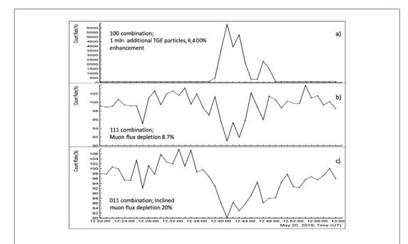
**Figure 3:** Extreme TGE event detected by SEVAN detector located on Musala mountain: a) – TGE particles – electrons and gamma rays; b) high energy muons; c) inclined muons, first published in: Phys. Rev. D 103, 043021, DOI: https://doi.org/10.1103/PhysRevD.103.043021.
