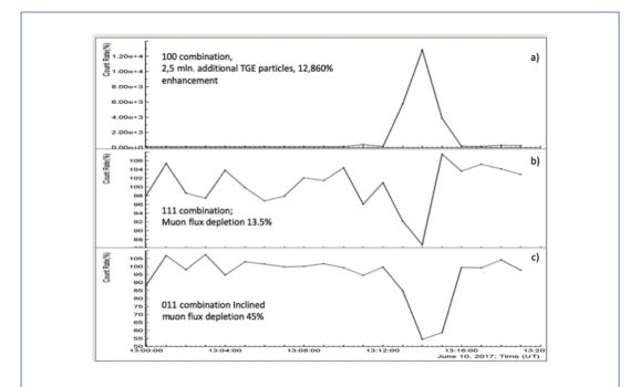
**Figure 2:** Extreme TGE event detected by SEVAN detector located on Lomnický štít mountain: a) – TGE particles – electrons and gamma rays; b) high energy muons; c) inclined muons, first published in: Phys. Rev. D 103, 043021, DOI: https://doi.org/10.1103/PhysRevD.103.043021.
