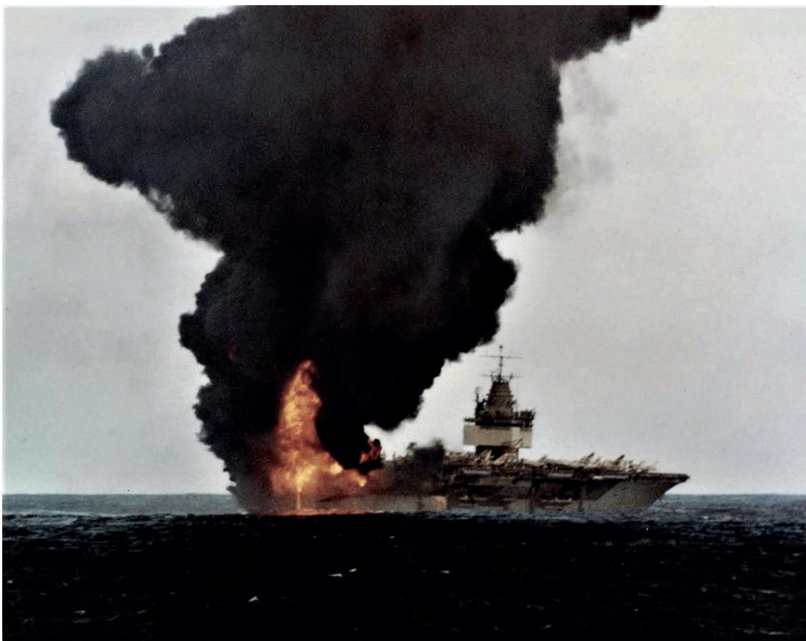
Fig. 26: The USS *Enterprise* is burning off the coast of Hawaii, 14 January 1969. The conflagration was set off by an accidental warhead detonation of a 5-inch unguided rocket on the flight deck and quickly turned into the third major munitions fire aboard an attack carrier in as many years. (U.S. Navy)
