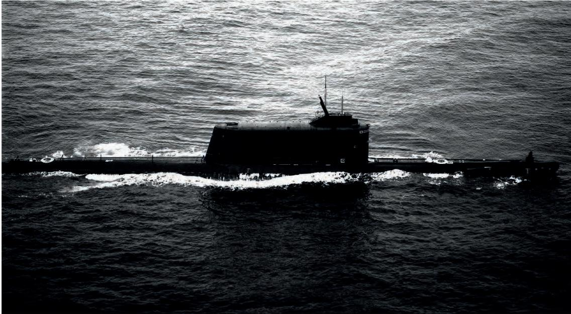
Fig. 16: Like its *Hotel*-class nuclear counterpart, the *Golf*-class carried three ballistic missiles in its elongated sail. After the switch to longer-range missiles and a much larger, Western-style missile battery in the *Yankee*, these early ballistic missile submarines were reassigned to the theater nuclear strike mission. (U.S. National Archives)
