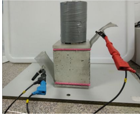
Figure 3.5.: Setup for electrical resistivity measurement (CSIC, Spain).
