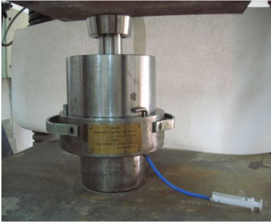
Figure 3.4.: Setup for pore pressing method test (CSIC, Spain).
