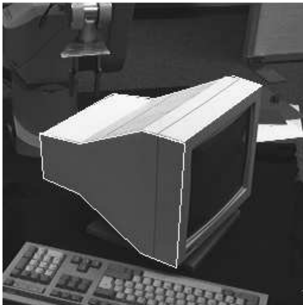
FIG. 25: Computer monitor with two types of regularities of the polygonal faces. The side face is approximate reflection-symmetric, and the top face is approximate translation-symmetric.
