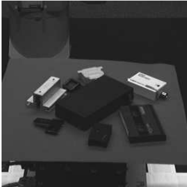
FIG. 15: Arrangement of objects in a scene of electrical scrap. The black dummy box is our target object for the purpose of demonstration. It is located in a complex environment, is partially occluded, and has a protruding socket.
