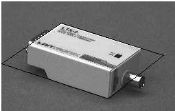
FIG. 38: Transceiver box with approximate right-angled parallelepiped shape. The black quadrangle surrounding the object indicates the image window for detailed processing.
