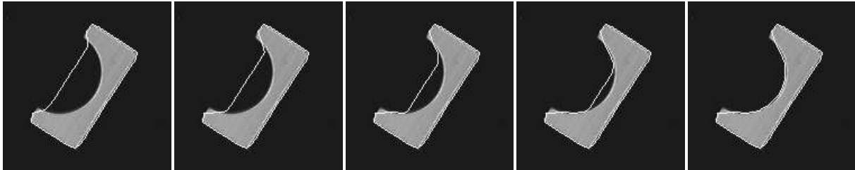
Figure 10: Minimization of the included area, starting with a polygon similar to the end polygon in figure 9 but with equidistantly distributed points.
