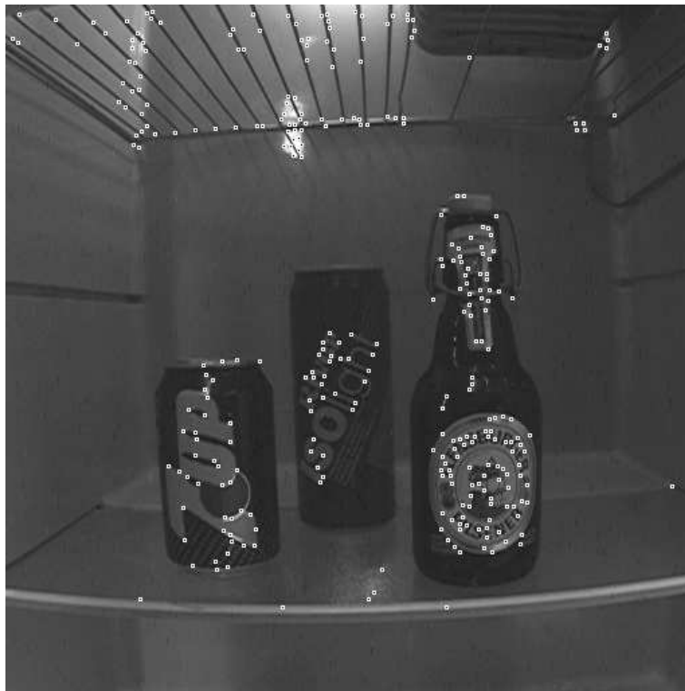
Figure 25: Detected grey level corners at two obstacle objects (left and right) and one goal object (middle).
